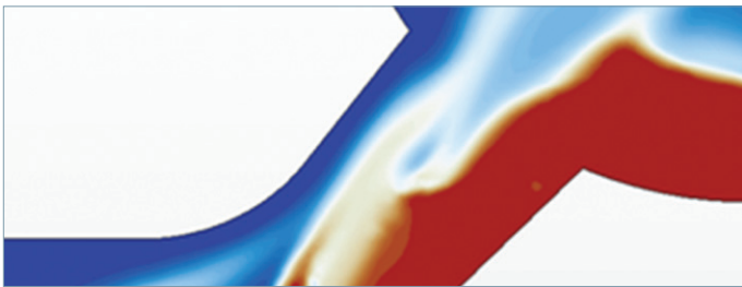
Figure 2. Stratified flow with liquid interface breakup and entrainment.
