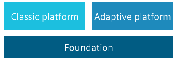
Figure 4. The Foundation standard of AUTOSAR provides functionality needed in both the Classic and Adaptive platform versions.
