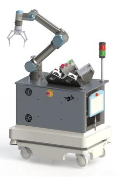
**LiDAR sensors** are ubiquitous across both AGV and AMR platforms, but not all systems are run the same way. For AGVs, lidar sensor simulations are used to define the position for reflectors within the work area, whereas AMRs require a virtual scan of the shop floor. There is also detection range planning that must be done virtually, such that the mobile platforms can navigate the floor without tripping a fail-safe function.
