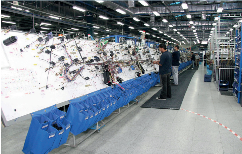
Figure 5: The formboard provides a full scale drawing of the harness to aid in manufacturing
