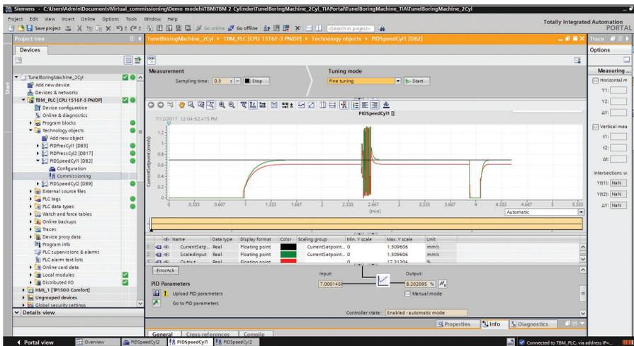
transient dynamics of multidomain systems directly coupled with the automation program (SiL) or the real programmable logic controllers (HiL). Typically, the impact of a programmable logic controller (PLC) code modification on the overall or energetic-only performance can be quickly and efficiently evaluated before the physical equipment exists. This increases flexibility and reduces development risks.
