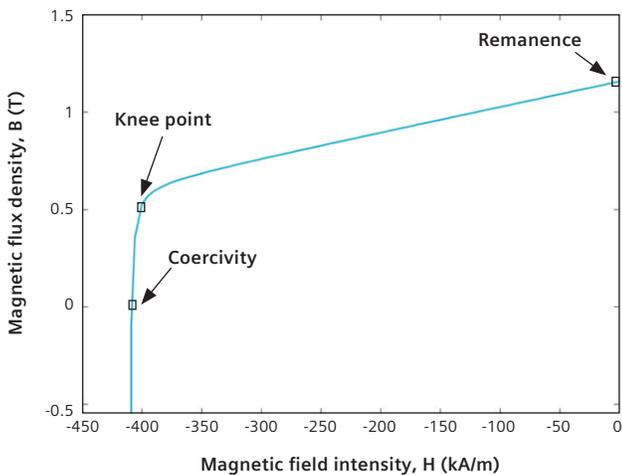
Figure 1: Measured Demagnetization BH curve of a high coercivity NeFeB magnet (N42) at 120 °C.
