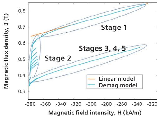
Figure 13: Test case 1c – BH plot for the N42 permanent magnet in the magnetization direction.
