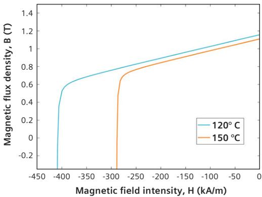
Figure 14: Measured demagnetization BH curves of the N42 permanent magnet at 120 °C and 150 °C.
