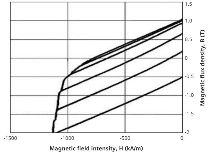
Figure 2: Measured recoil curves of a high coercivity NeFeB magnet at 120 °C [2].
