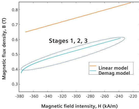
Figure 11: Test case 1b – BH plot for the N42 permanent magnet in the magnetization direction.
