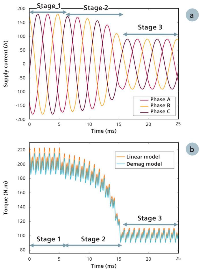
Figure 9: Test case 1b (a) Supply current (b) Torque using the linear and the Demag models.
