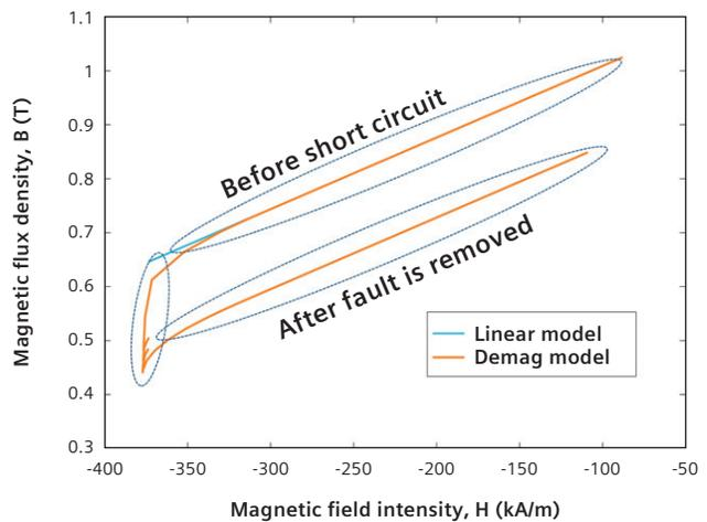
Figure 19: Test case 3 – BH plot for N42 permanent magnet during short circuit fault in the magnetization direction.
