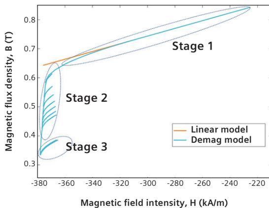
Figure 8: Test case 1a – BH plot of the N42 permanent magnet in the magnetization direction at a field sample point.
