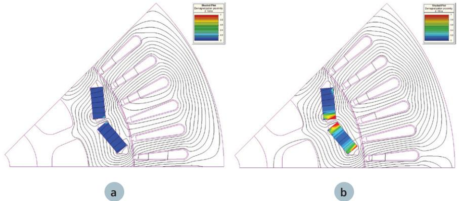
Figure 16: Test case 1a – Sample Demagnetization Proximity plots for the N42 permanent magnet at 10 ms for (a) 120 °C (b) 150 °C.
