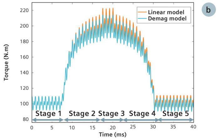
Figure 12: Test case 1c (a) Supply Current (b) Torque using the linear and the Demag models
