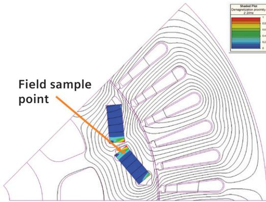
Figure 10: Demagnetization Proximity plot using the Demag model for the N42 permanent magnet at 0 ms at a field sample point.
