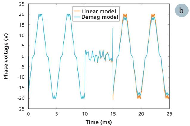
Figure 18: Test case 3 (a) Phase current during short circuit (b) EMF – Phase voltage using the Demag and linear models.
