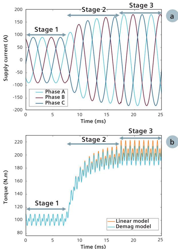
Figure 6: Test case 1a (a) Supply current (b) Torque using the linear and the Demag models.
