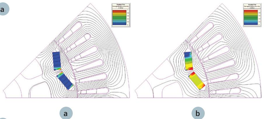
Figure 17: Test case 1a – Demagnetization Proximity plots for the N42 permanent magnet at 20 ms for (a) the linear model at 120 °C (b) the Demag model 150 °C.
