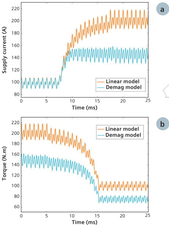
Figure 15: Test case 2 – Torques computed using the linear and the Demag models at 150 °C for (a) Test case 1a, and (b) Test case 1b.
