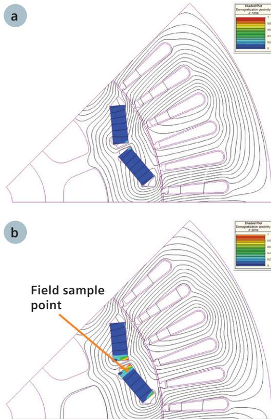
Figure 7: Demagnetization Proximity plots for N42 permanent magnet for (a) the linear model at 10 ms (b) the Demag model at 20 ms.
