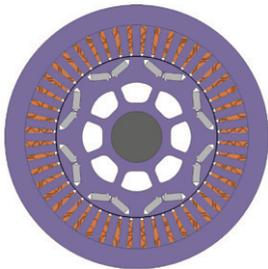
Figure 5: Simcenter MAGNET model of the IPM motor.
