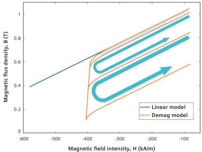
Figure 4: BH plot for an N42 permanent magnet using the linear and the Demag models in the magnetization direction.
