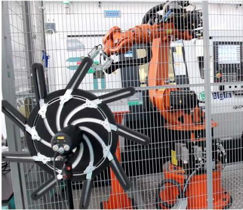
Localizing sound sources and vibration of an industrial robot
