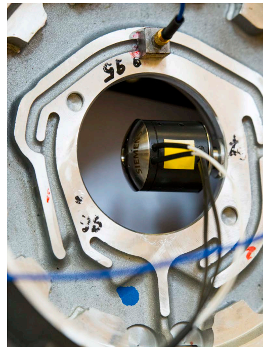
Regardless of location, quickly measure accurate transfer functions with the self-aligning Simcenter QSource miniature shaker.
