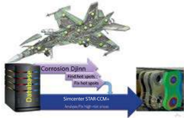
Figure 3: Corrdesa corrosion analysis engineering workflow
