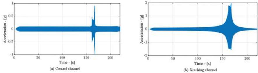
Figure 8: Control and notching channel in time domain
