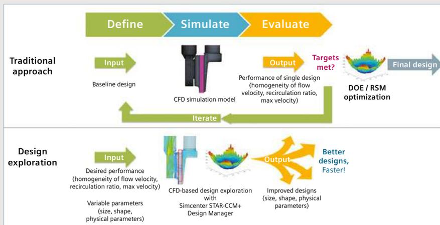
Figure 3: Traditional design approach versus design exploration.
