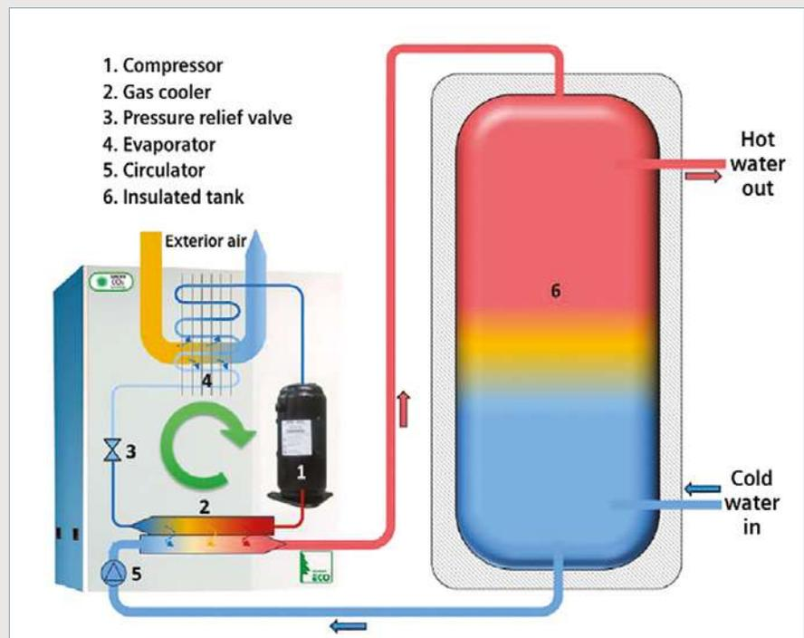
Figure 1: Schematic of a CO<sub>2</sub>-based air/water heat pump.
