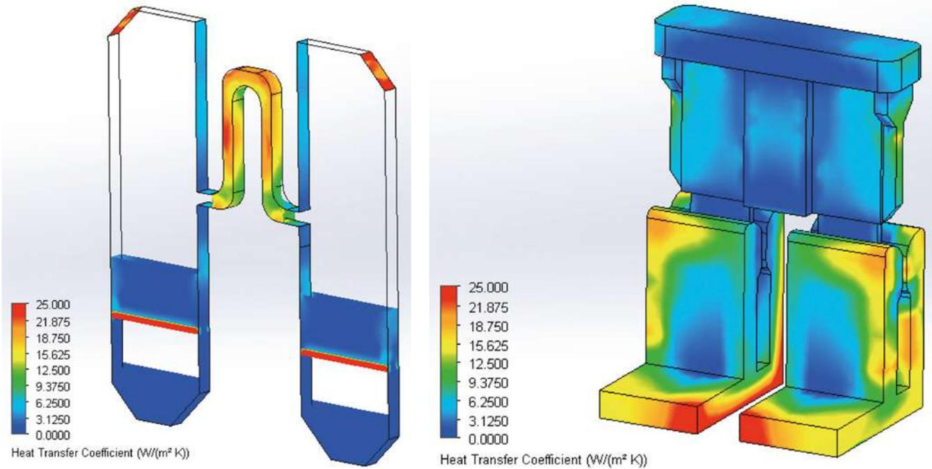
Figure 4: Local surface heat transfer coefficients on blade-type automotive 10A fuse
