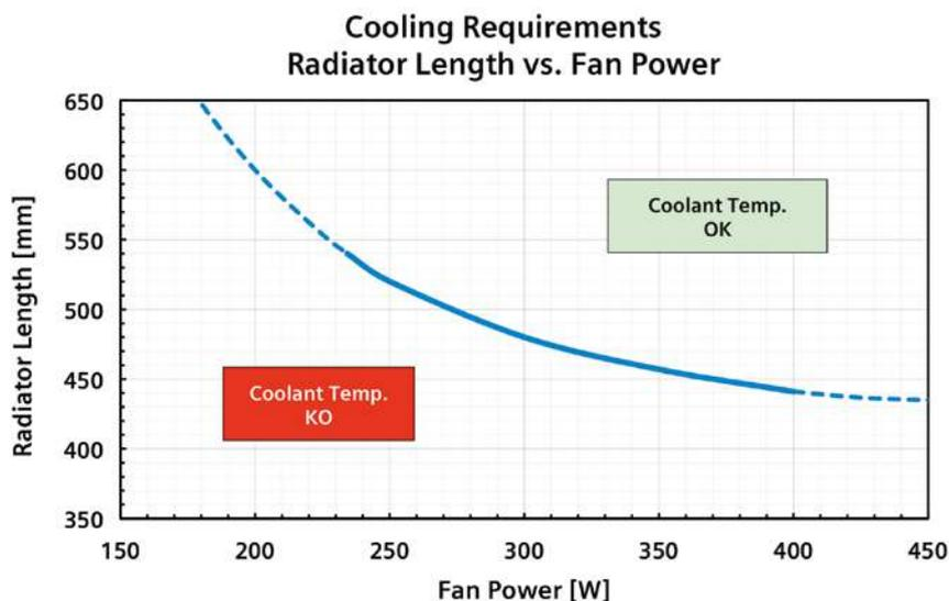
Figure 8: Cooling requirements according to all driving conditions
