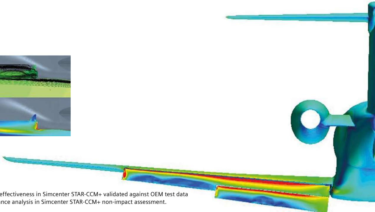
Figure 5: (Left) Flap effectiveness in Simcenter STAR-CCM+ validated against OEM test data (Right) Cavity resonance analysis in Simcenter STAR-CCM+ non-impact assessment.
