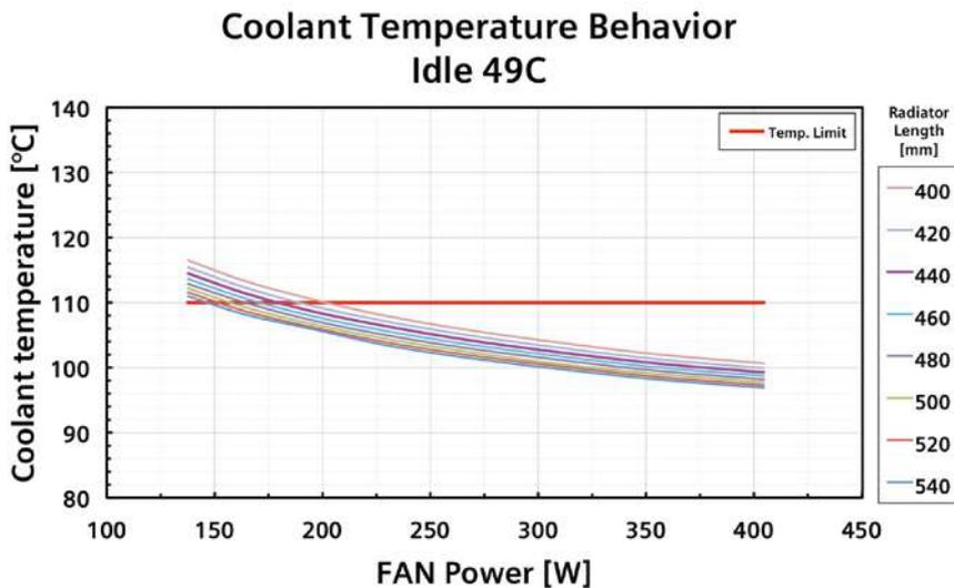
Figure 7: Coolant temperature drive scenario G test case
