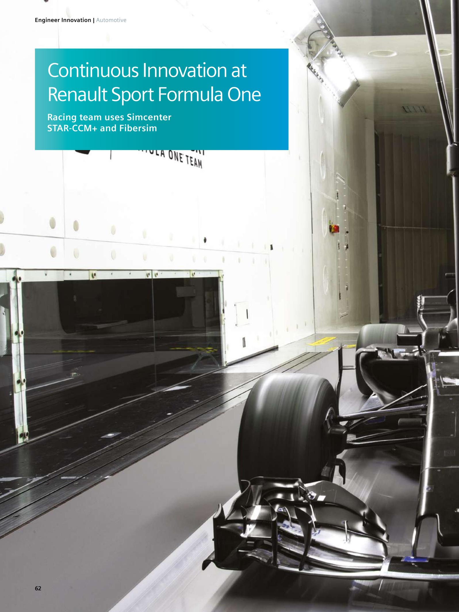
Driving with downforce, drag and danger. The dynamic between grip and drag dictates design preparation for each race in the Formula One calendar. A large rear wing creates the downforce required for tight cornering at Monaco. For Monza, where too much downforce would slow the car on fast straights, a slender rear wing is needed.
