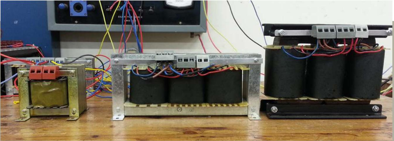
Figure 1. Bench-scale transformers single-phase shell type (left) three-phase five limb (centre) and three-phase three limb (right).
