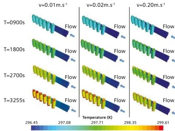
Figure 2: The temperature rise in the first set of series cells in the pack is a function of the 0.9 (°C) discharge rate and contact resistance of 0.0025 (m<sup>2</sup>.°K)/W.
