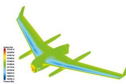
Figure 2: Mach No. contour and surface pressure distribution at Velocity = 50 mph, Angle of Attack= 0°.
