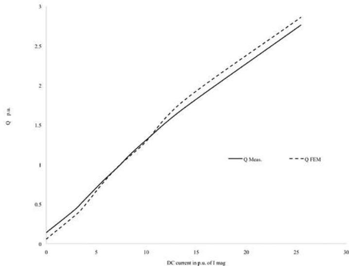
Figure 3. Measured and simulated reactive power Q in per unit (p.u.) of the VA rating vs. DC in p.u. of the transformer magnetizing current (I<sub>mag</sub>) for 1p3L laboratory transformer.
