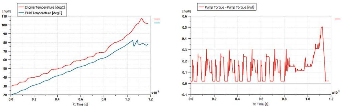
Figure 4: Simcenter Flomaster provides Simcenter Amesim with values of engine temperature, fluid temperature downstream of the engine and pump torque.
