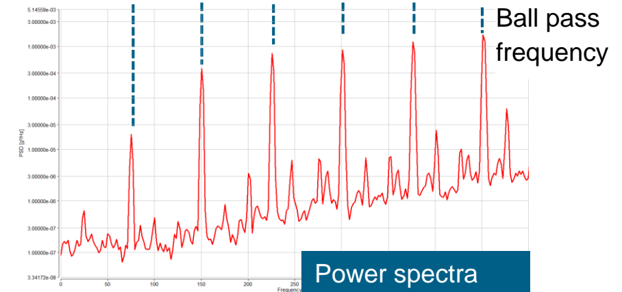
Example A: Bearing failure – Outer race damage
