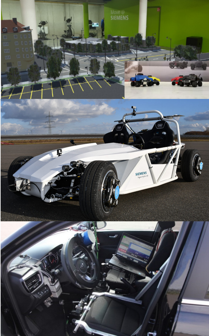
Figure 14: Different autonomous vehicle platforms: small vehicles with augmented reality (AR), Simrod vehicle, and conventional vehicle equipped with driving robots.
