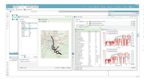
Simcenter Amesim 2019.1 to obtain a shared battery model. You can visualize parameters of the imported model before using them in Simcenter Amesim.
