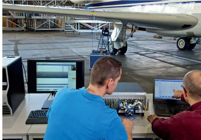
Ground vibration testing setup.
