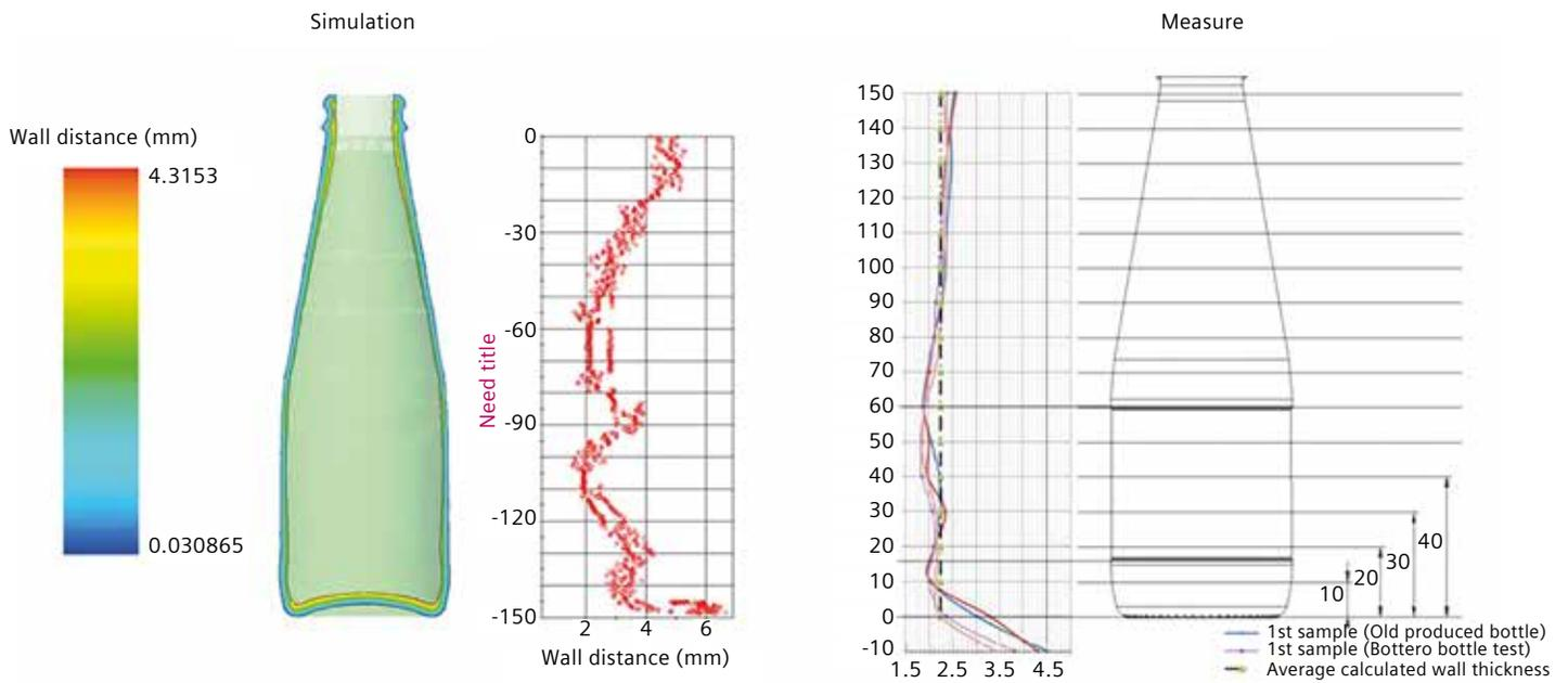
Figure 9: Validation of numerical simulations with Simcenter STAR-CCM+ showing good comparison when comparing wall thickness to real bottles.
