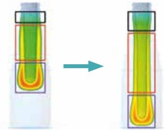
Figure 7: Simulation with Simcenter STAR-CCM+ showing the shape change of the parison in the blow mold.
