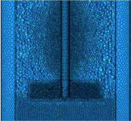
Figure 2: Polyhedral mesh in the computational fluid domain of the vessel and HTPG4 impeller using Simcenter STAR-CCM+.
