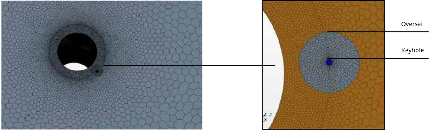
Figure 1: One of the unique features of Simcenter STAR-CCM+ that Bemis found extremely useful was overset mesh, a major advance in simulation.
