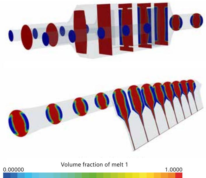
Figure 4: Progressive volume fraction at sections: injector block (top) and end fed die (below).
