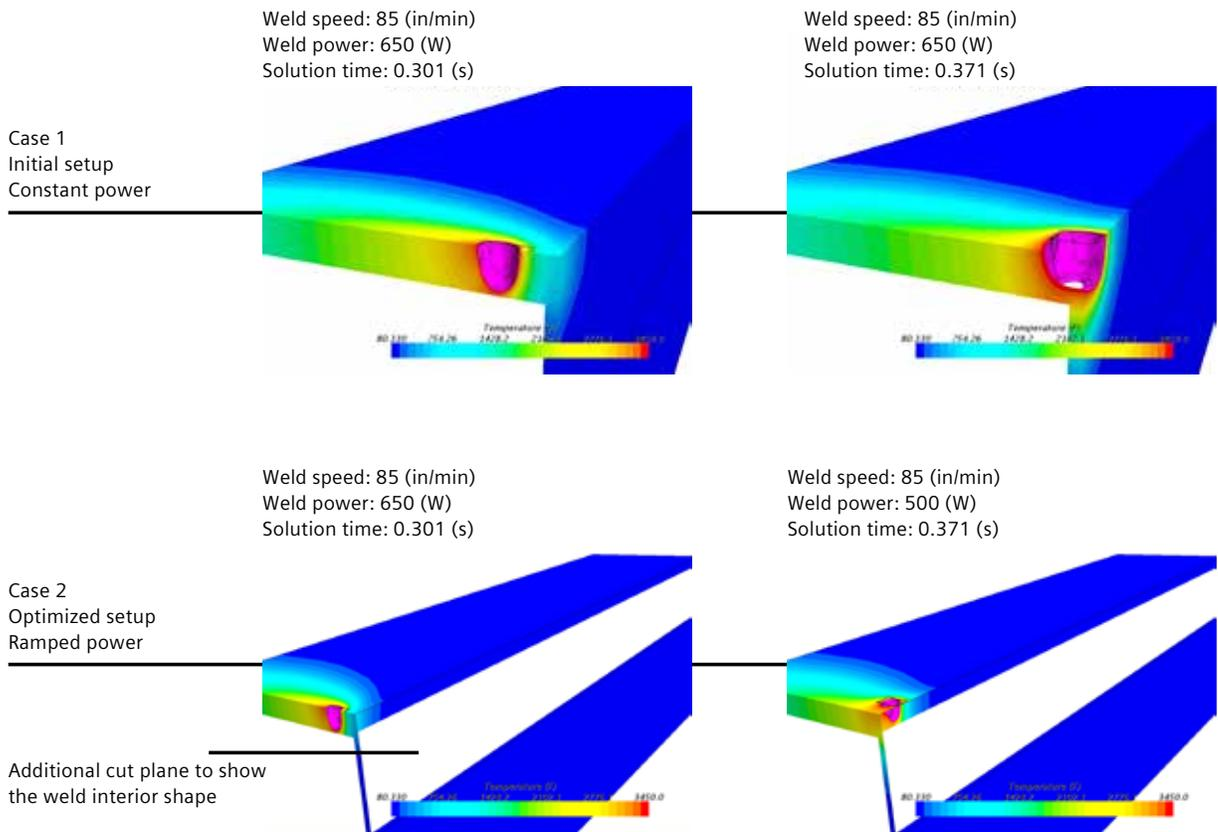
Figure 5: Case 1 shows how weld pool melts through the corner at constant power and speed. Case 2 pictures an optimized setting allowing for a uniform melt pool throughout the weld cycle.
