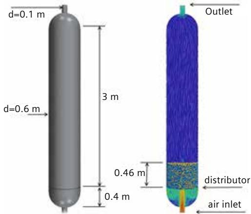
Figure 1: Geometry and boundary conditions for riser study.
