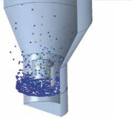
Figure 3: DEM simulation for tablet coating thickness in a fluidized bed.
