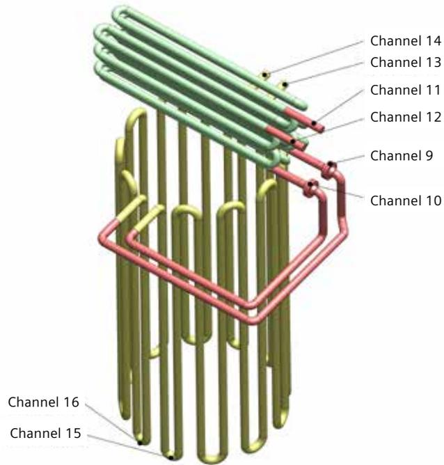
Figure 2: Locations of accelerometers on the test system.
