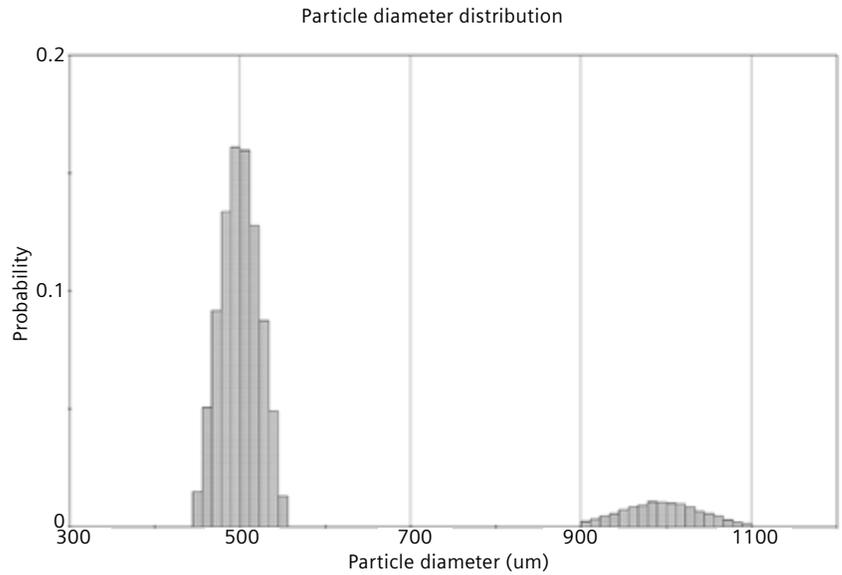
Figure 2: Size distribution of particles: fines with a distribution clustered around 500 microns and coarse particles around 1 mm.
