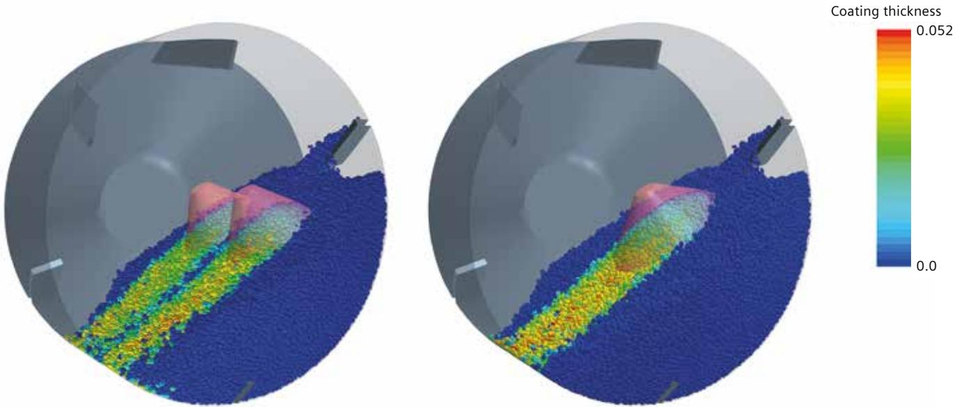
volume confined to two cones and with an effective spray area identical to the one of the first passive scalar. Using this approach, a single simulation allows for a comparison of the interparticle coating uniformity for two different spray zones and the result indicates the two-spray configuration provides a more uniform coating distribution.
