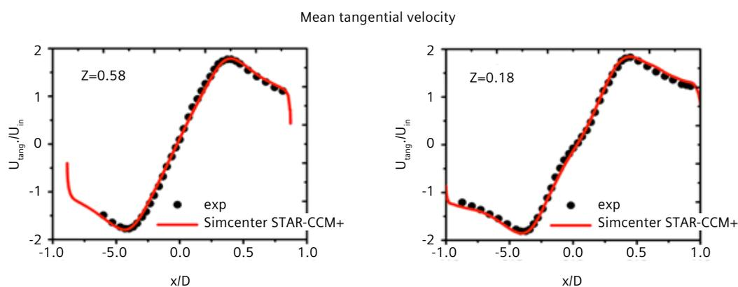
Figure 10: Average tangential velocity at two cross sections of the cyclone: CFD compared to experiment.
