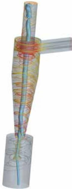
Figure 7: Streamlines showing the separation of heavy particles (lower outlet) and light particles via the central vortex.
