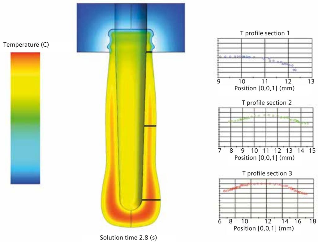
Figure 3: Parison temperature during reheating showing temperature redistribution.
