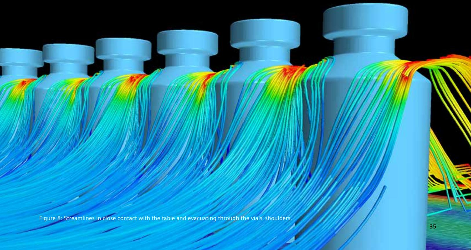
Figure 8: Streamlines in close contact with the table and evacuating through the vials' shoulders.
