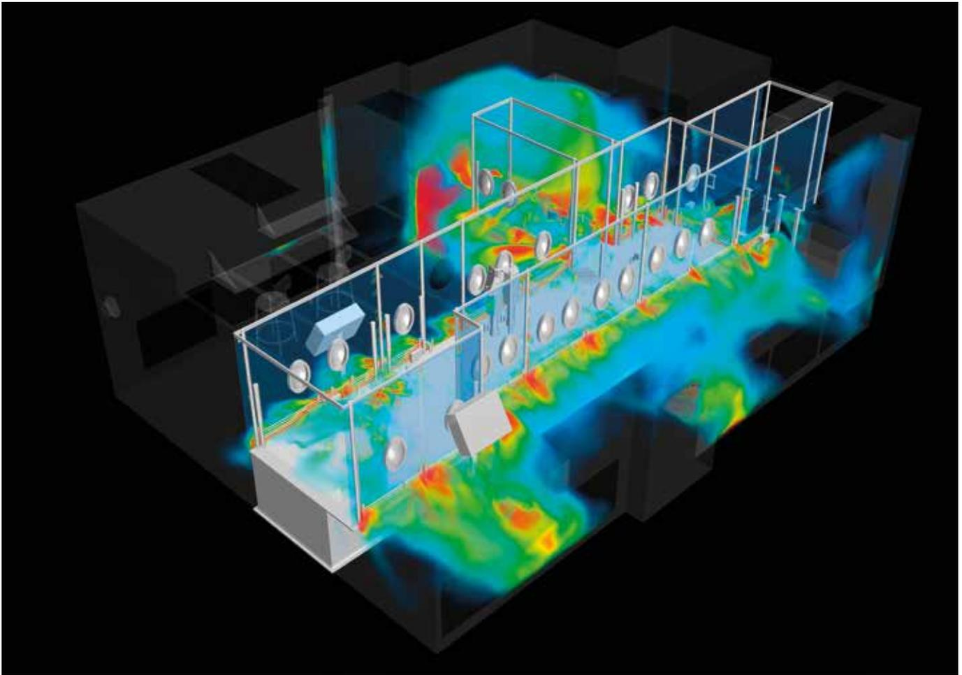
project, Laporte was in charge of the process design, installation and commissioning for the pharmaceutical facility upgrade. These tasks include the HVAC design and the integration of the filling machine in the RABS system. Laporte was also responsible for the preliminary smoke tests used for regulatory compliance.
