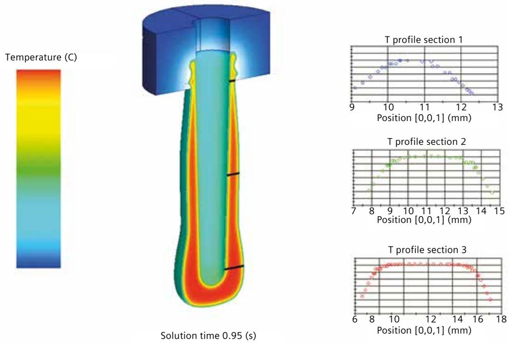
Figure 2: Detailed 3D temperature model of the parison showing realistic vertical temperature trends.
