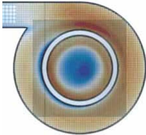
Figure 6: Cross sectional view of the cyclone geometry, mesh and contours of tangential velocity.
