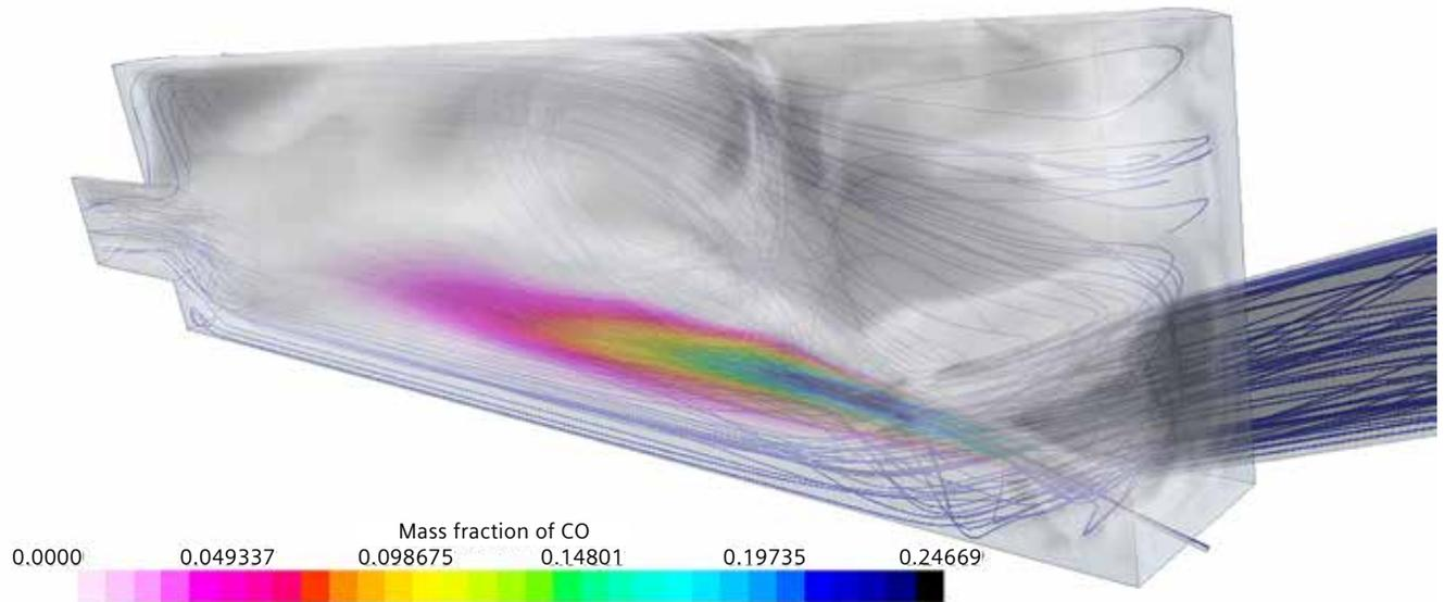
Figure 9: CO mass fraction field in glass furnace simulation using the FGM combustion model.
