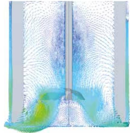
Figure 3: Velocity vectors and power number.
