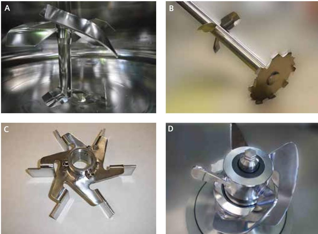
Figure 1: Different types of impellers manufactured by Pierre Guerin: (A) Low shear HTPG4 propeller for cell cultivation; (B) Heli Turbo Agitator HTA for powder dispersion; (C) Rushton turbines for aerobic fermentation; (D) Magnetic mixer PG-MAG for ancillary vessels.
