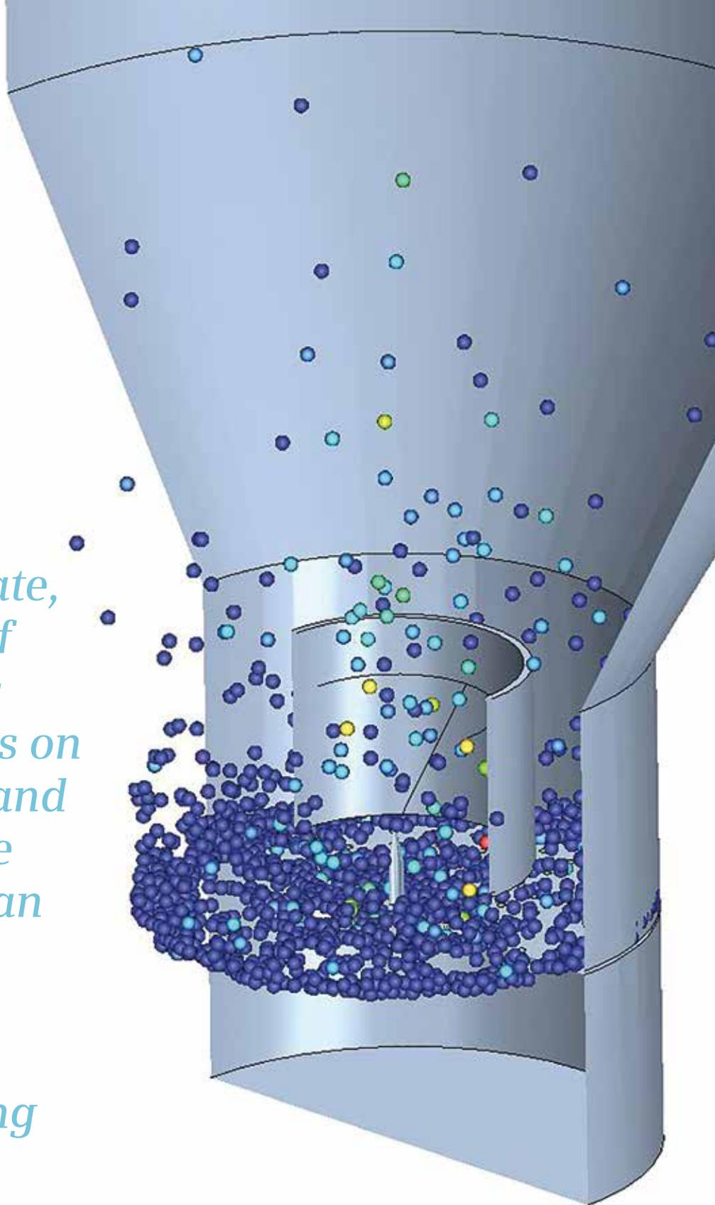
Figure 2: Simcenter STAR-CCM+ simulation of the coating process performed in a fluidized bed.
