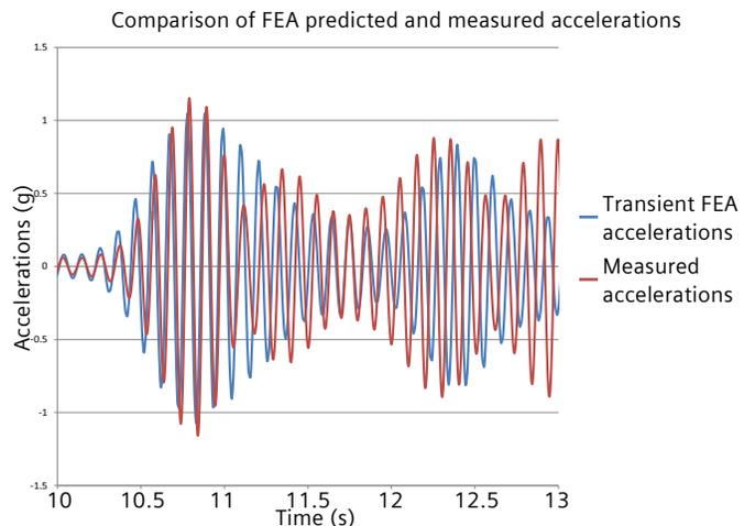
Figure 8: Comparison of FEA-predicted accelerations and measured accelerations.
