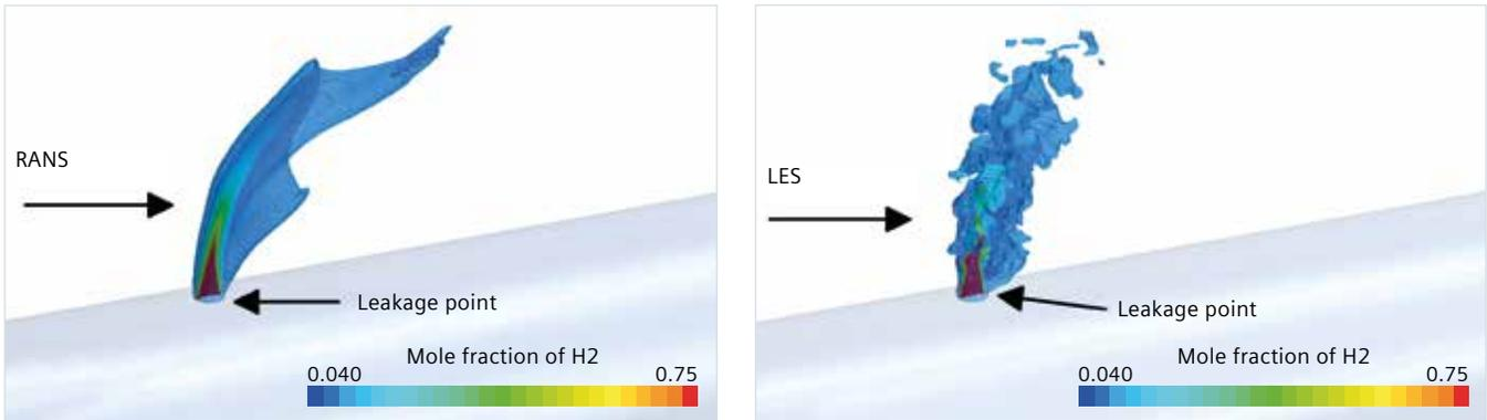
Figure 3: Hydrogen leak diffusion analysis using RANS (left) and LES (right) in Simcenter STAR-CCM+.
