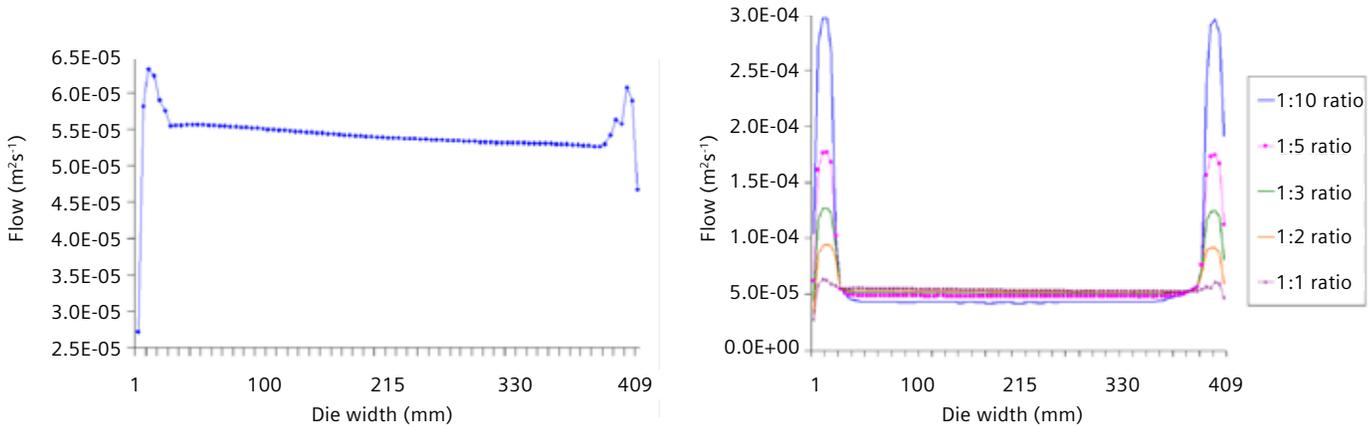
Figure 9: Flow across the outlet for 1:1 viscosity ratio (left) and flow across outlet for increasing ratios (right) for MMD.
