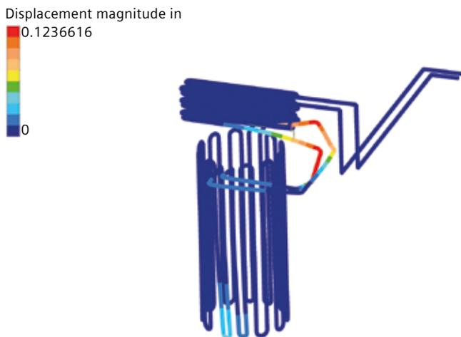
Figure 7: CFD calculated displacement of flow pipe, accurately predicting locations of heaviest vibrations.
