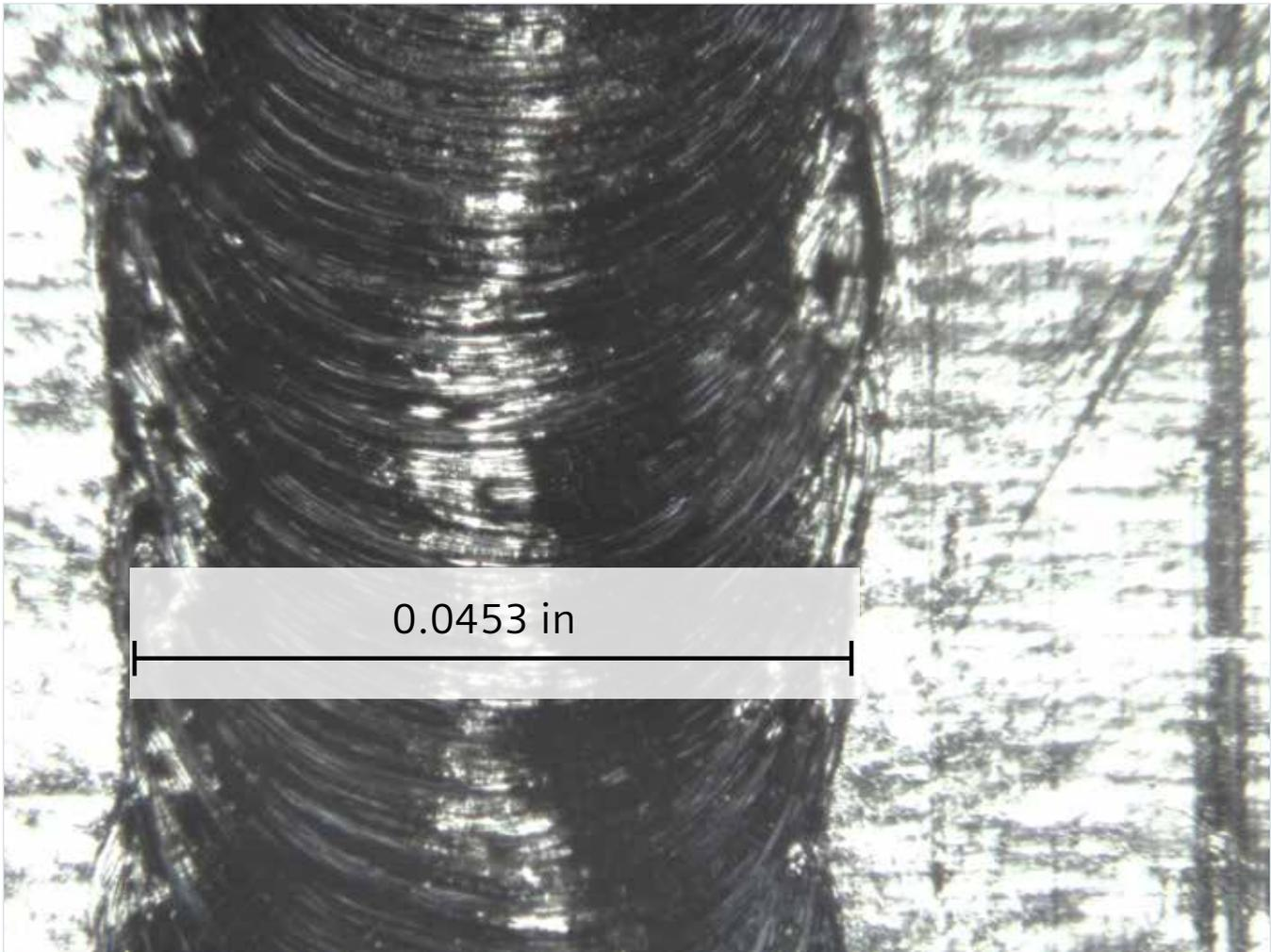
Figure 6: Validation of weld zone width and depth was done using optical microcopy.
