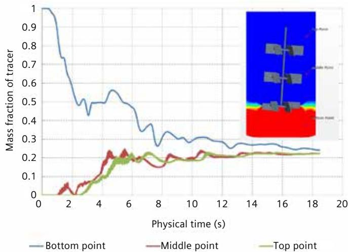
Figure 1A: Inert tracer method (resembling the widely used experimental technique) showing the quantitative change in local concentration as a function of time.
