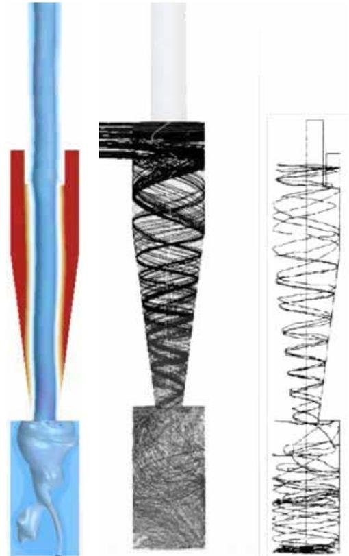
Figure 8: Snapshot of vorticity down the cyclone centerline, and particle trajectories – CFD (left) and experiment (middle and right).
