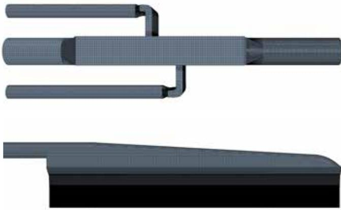
Figure 3: Mesh on the injector block and end fed die.
