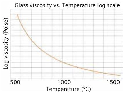
Figure 6: Variation of glass viscosity with temperature during the glass forming process.
