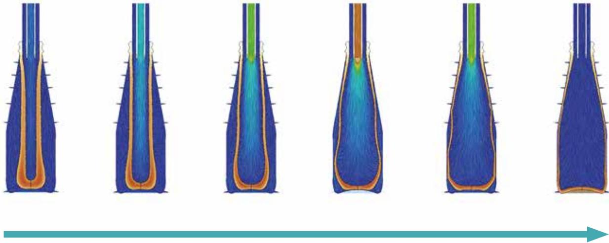
Figure 8: Complete simulation with Simcenter STAR-CCM+ for the glass forming process, starting from the initial glass gob to the final shape.
