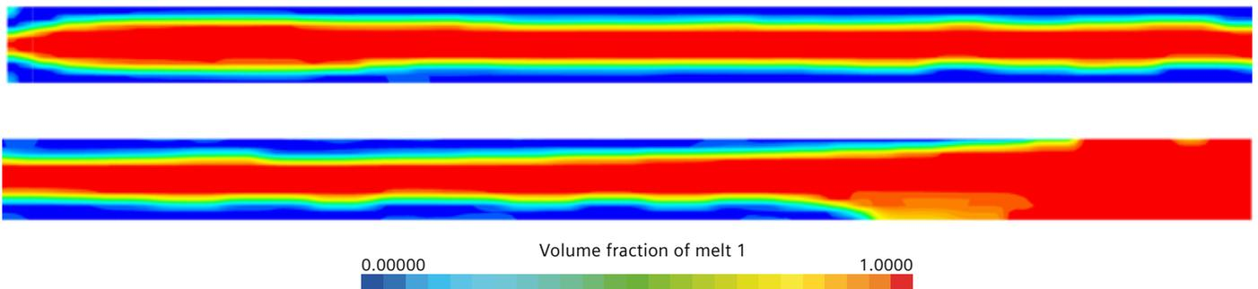
Figure 5: Volume fraction at outlet for injector block and end fed die.
