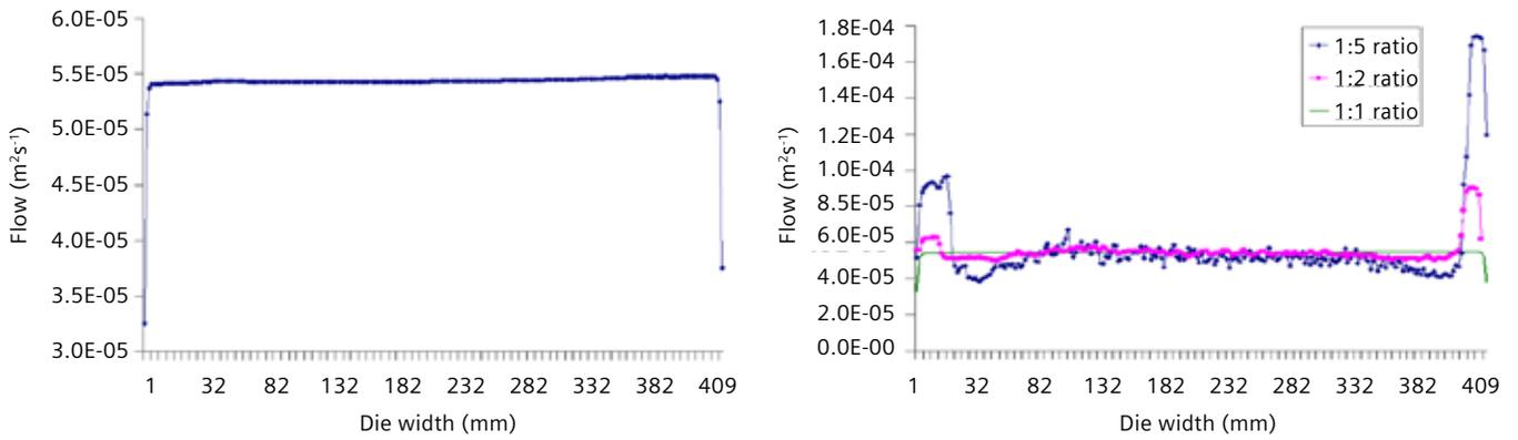
Figure 6: Flow across the outlet for 1:1 viscosity ratio (left) and flow across outlet for increasing ratios (right).
