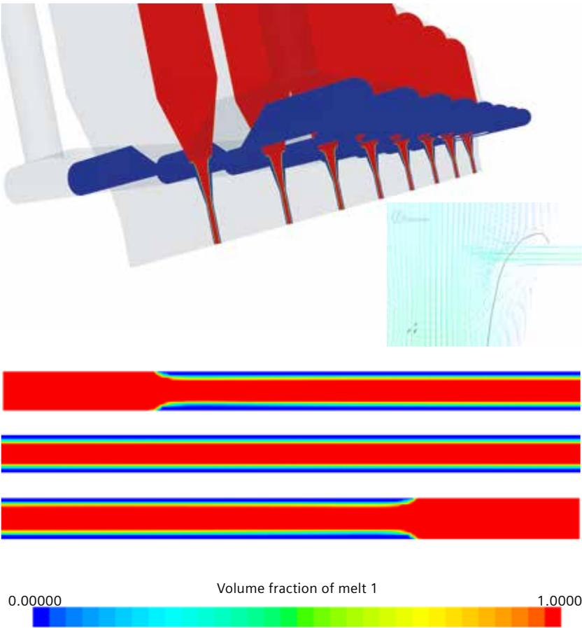
Figure 8: Progressive volume fraction (top) and outlet volume fraction (bottom) in MMD.
