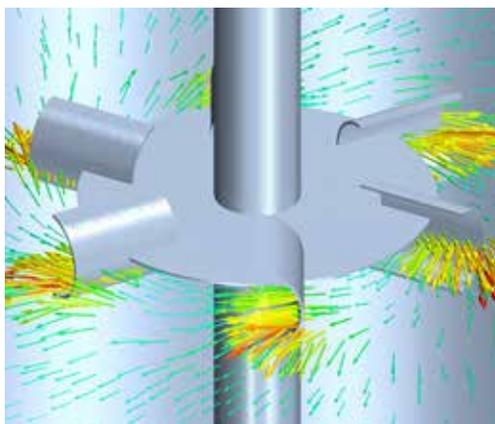
Figure 3: Predicted 3D flow pattern around impellers of a mixing tank using Simcenter STAR-CCM+.
