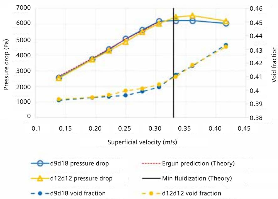
Figure 5: Mean pressure drop and void fraction against superficial velocity.
