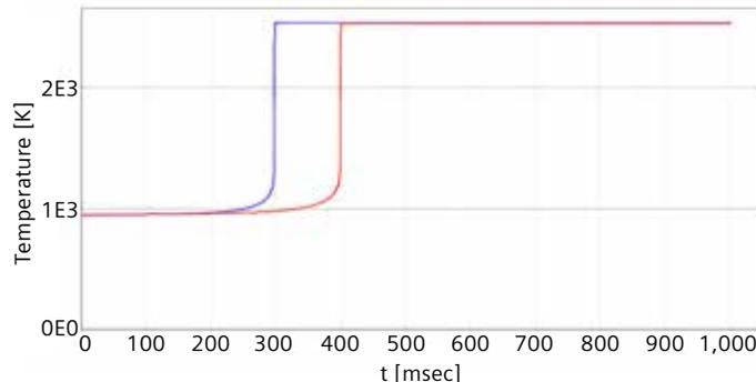
Figure 4: Ignitability for different natural gas qualities at initial temperature of 950K (red line: high quality, blue line: low quality).
