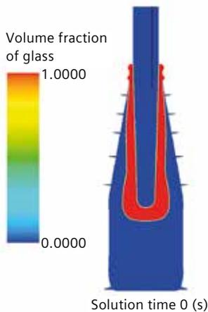
Figure 5: Volume fraction of glass in the dynamic model of the parison for simulating shape changes.
