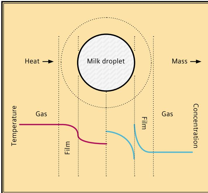
Drying process in a spray dryer (heat and mass transfer).
