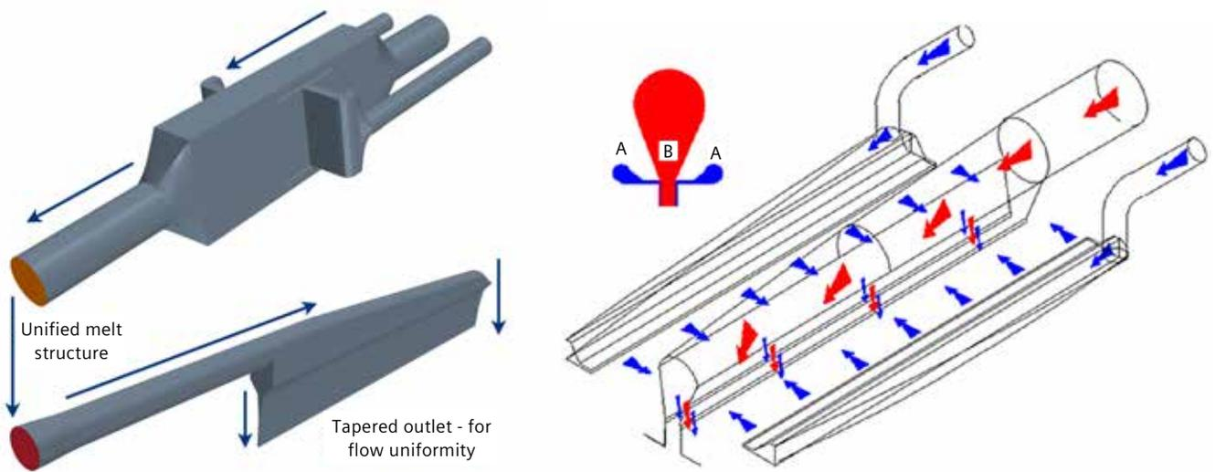
Figure 2: Common DTF coextrusion structures: injector block and end fed die (top) and multi-manifold die (bottom).
