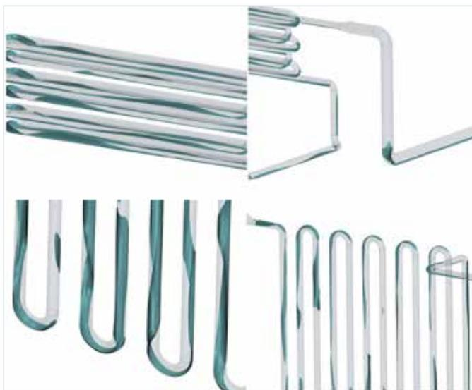
Figure 6: CFD calculated flow of liquid in the pipes, showing heavy slugging.
