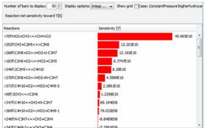
Figure 7: Reaction sensitivities for low-quality natural gas combustion.
