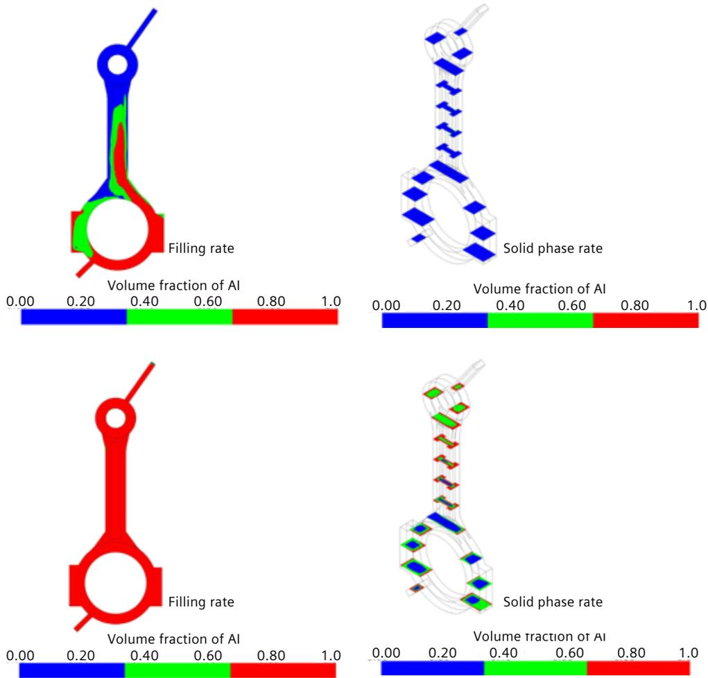
Figure 2: Cast part fluidity and solidification analysis using Simcenter STAR-CCM+ showing filling rate and solid phase rate during casting (above) and post-casting solidification (below).
