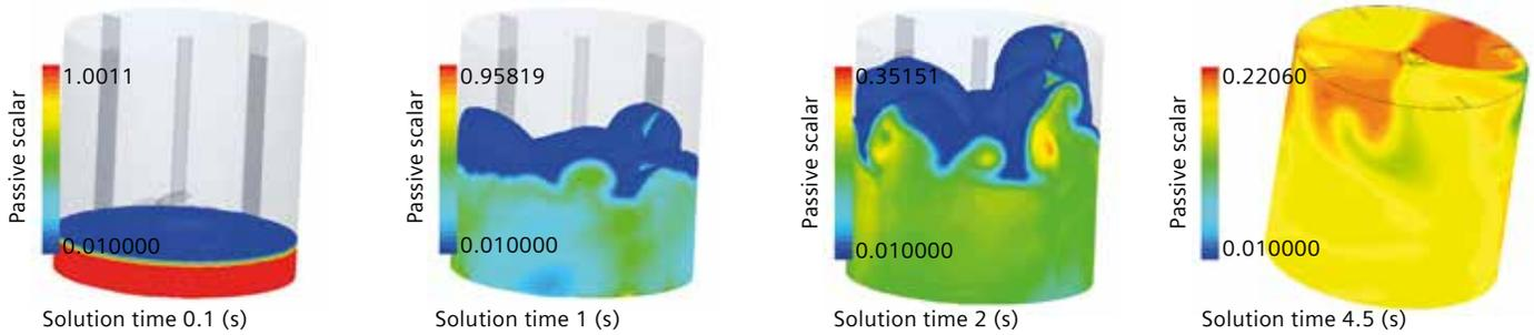
Figure 4: Time evolution of the passive scalar.
