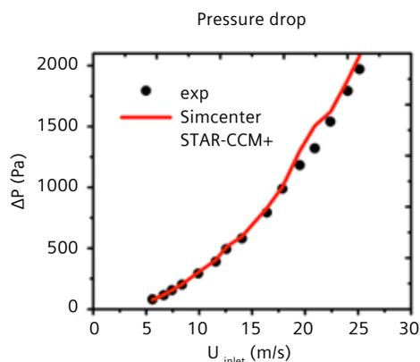
Figure 9: Average pressure drop across the cyclone versus inlet velocity: CFD and experiment.
