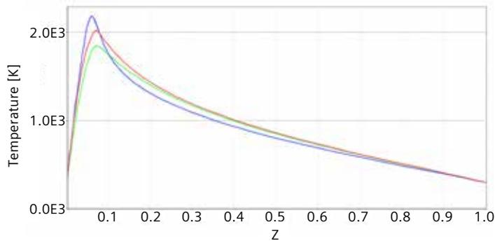
Figure 3: Flamelet temperature for low-quality natural gas for various scalar dissipation rates (green line: very low scalar dissipation rate; blue line: very low scalar dissipation rate; red line: medium scalar dissipation rate; green line: scalar dissipation rate very close to extinction).
