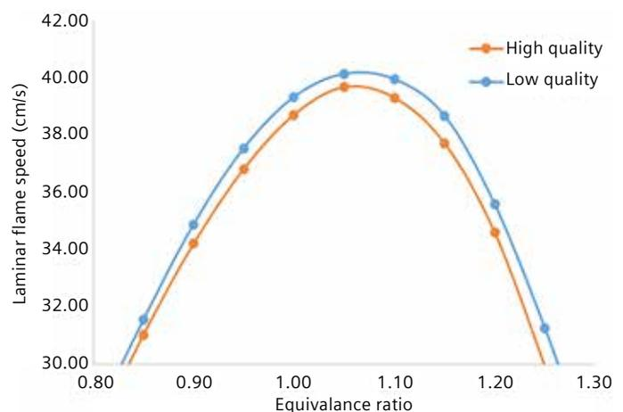
Figure 2: Laminar flame speed for high- versus low-quality natural gas.
