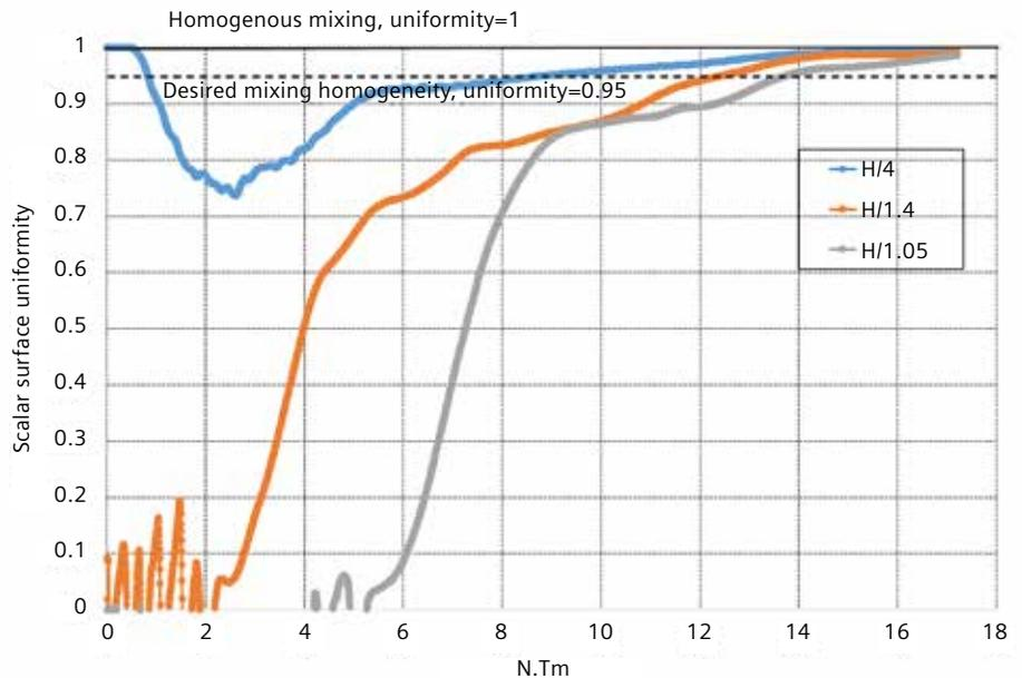
Figure 5: Time evolution of the passive scalar tracer concentration at different levels; dashed line on the graph indicates the desired mixing homogeneity (uniformity=0.95).
