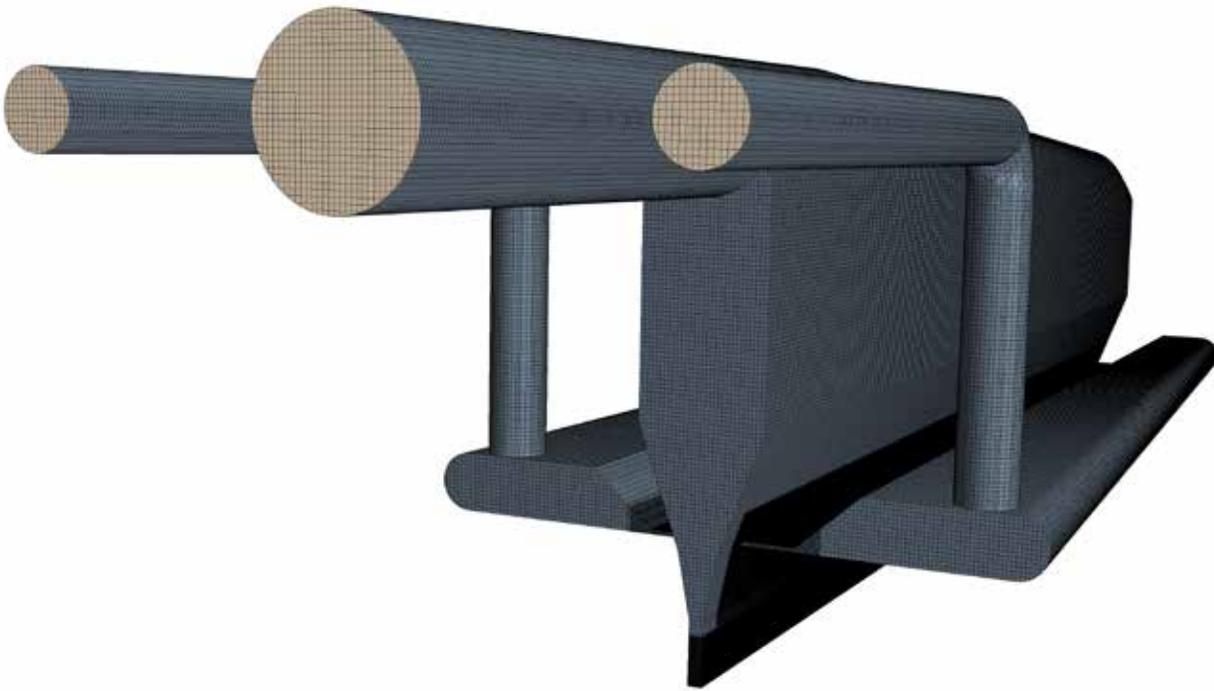
Figure 7: Mesh on multi-manifold die (MMD).
