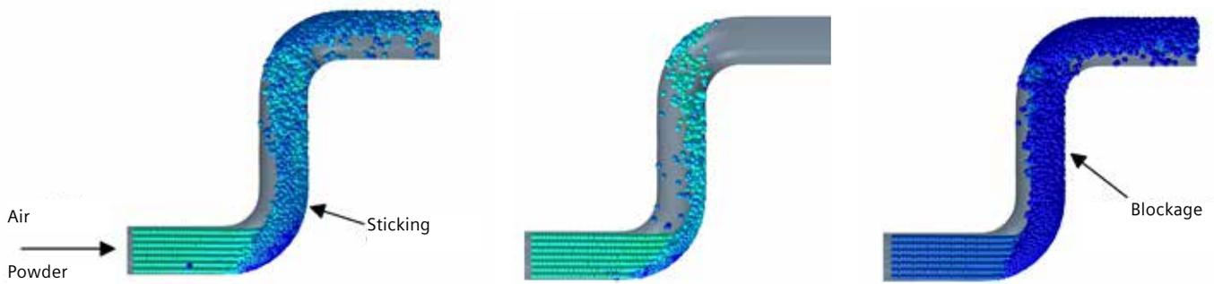
Figure 1: Powder behavior analysis in powder transport piping using Simcenter STAR-CCM+.
