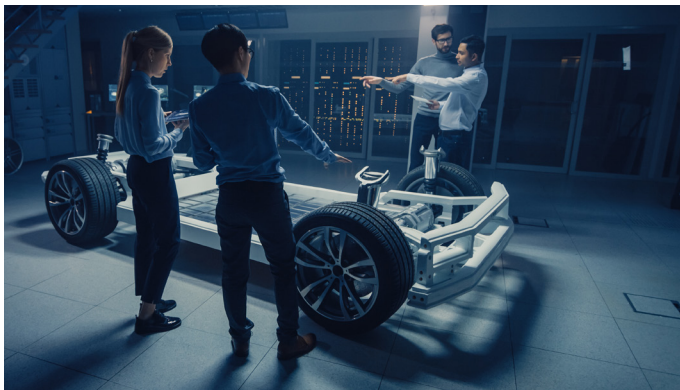
Figure 2: Native EV platforms provide more configuration flexibility and greater drive range by accommodating larger battery packs.
