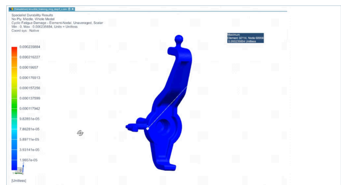
Figure 8: Maximum fatigue damage detection.
