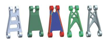
program know what you mean by optimal, you specify design and performance objectives for characteristics such as minimum weight, shape constraints and minimum stress or strain. Design parameters that you can vary include geometric, material and connectivity properties.
