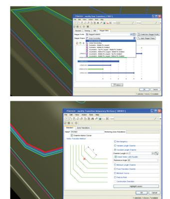
Fibersim zone transitions provide an automated way to create the desired drop-off profile by either using stagger shapes or dragging and dropping plies to the appropriate ply boundary.
