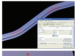
The Fibersim spine-based simulation is the only solution that allows you to identify areas of localized deformation (highlighted in yellow and red) that are caused by part curvature and fiber steering during manufacturing.
