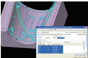
Fibersim manufacturing interfaces support myriad manufacturing processes, including automated cutting, automated fiber placement, automated tape laying and laser projection.
