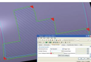
The Fibersim machine database and its course challenge detection simulation allow you to identify design issues due to automated fiber placement and automated tape laying machine characteristics, including minimum courses (highlighted in red) and shallow cut angles.
