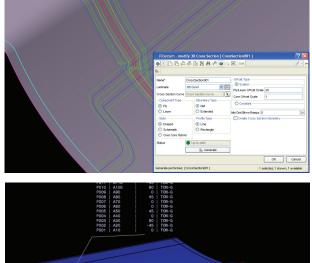
Fibersim cross sections are automatically created with a push button operation and are associative to the design, eliminating manual effort and ensuring accuracy.
