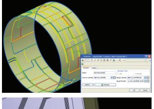
Fibersim parametric surface offset capabilities make it easy to create IML tooling (tan surface) and update it with design changes. The skin transfer capability automatically transfers the plies from the design definition (blue, yellow, green and red curves) to the manufacturing model.
