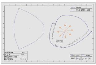
Fibersim generates plybook documentation needed for hand layup, which ensures repeatability and part quality by displaying the layup process.
