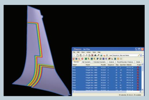
The Fibersim Excel import capability creates all of the plies from the imported Excel spreadsheet containing ply names, materials, orientations and CAD ply boundary names. Plies highlighted in Fibersim are displayed in the CAD model. Plies are indicated by blue-0°, green-45°, yellow-90°, red-45°.
