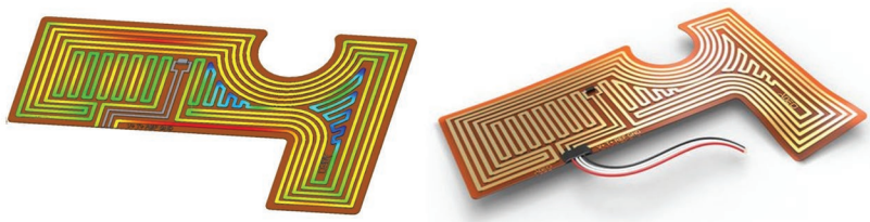
Figure 5. Example of a heater foil and thermal simulation showing temperature distribution (left) in detailed analysis (courtesy of ELINTER AG).
