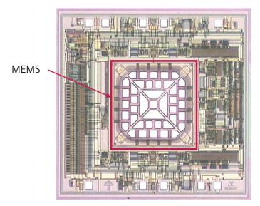
Figure 6: A MEMS device integrated on a CMOS IC. (Source: MEMSIC)
