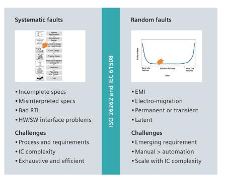
Figure 3: ISO 26262 requires that electronics are tested for systematic and random faults.
