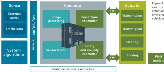
Figure 5: Hardware emulation can fuse sensor, compute and actuation data to create a testing environment for autonomous vehicle platforms.
