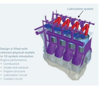
Figure 2: The virtual engine is brought to life with data from 1D simulation.
