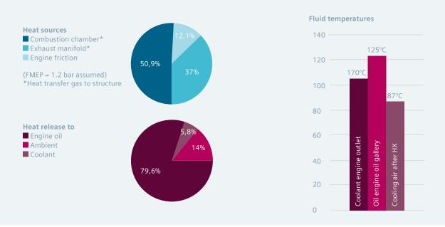
Figure 9: Breakdown of heat sources and where the heat is released in the Pandora model.
