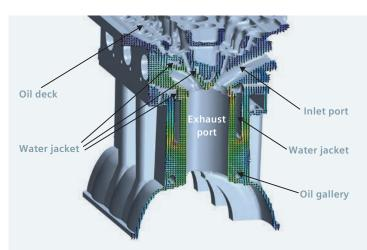
Figure 5: Heat flux vectors in the engine structure.
