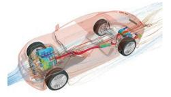
Figure 8: Streamlines through engine compartment for 240 KPH at 135 kW.
