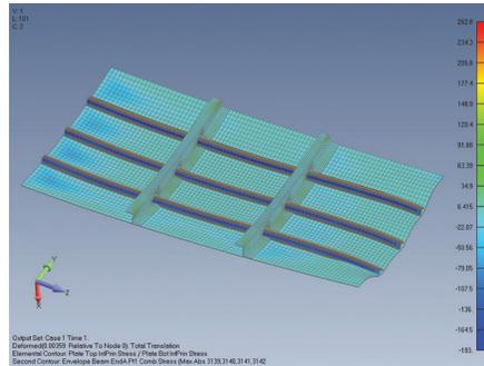
SOL 401 is the multi-step nonlinear solver where subcases can be dependent or independent of the previous subcase, and where you can change analysis type in a subcase. With this approach you can define linear, nonlinear, modal, and bolt preload subcases to create a combined solution in the analysis manager.
