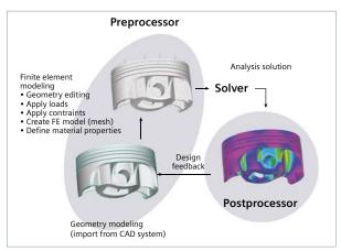
Figure 1: The finite element analysis process.
