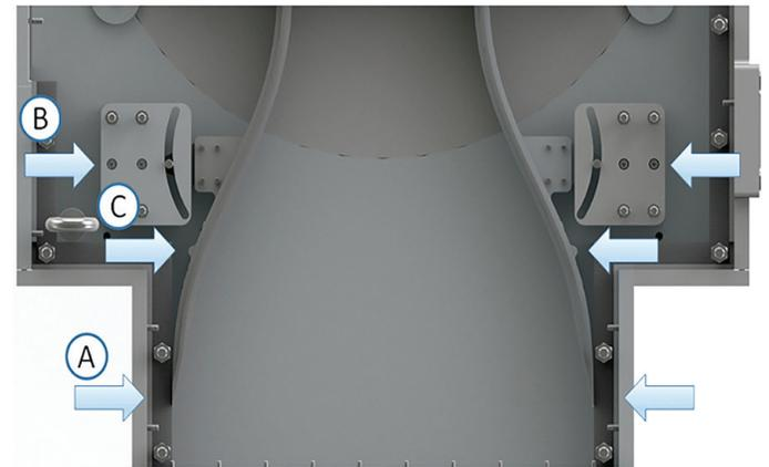
Figure 6: Frontboards sealing and support mechanisms.
