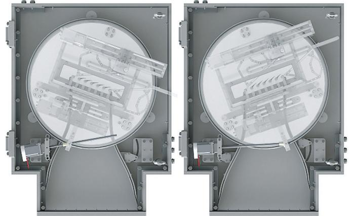
Figure 5: Disks rotation mechanism set to  $\pm 20^\circ$ .
