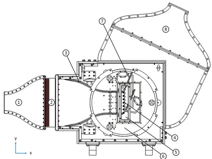
Figure 2: TTL test section layout and reference frame.
