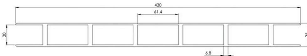
Figure 4: Turbulence grid design [mm].
