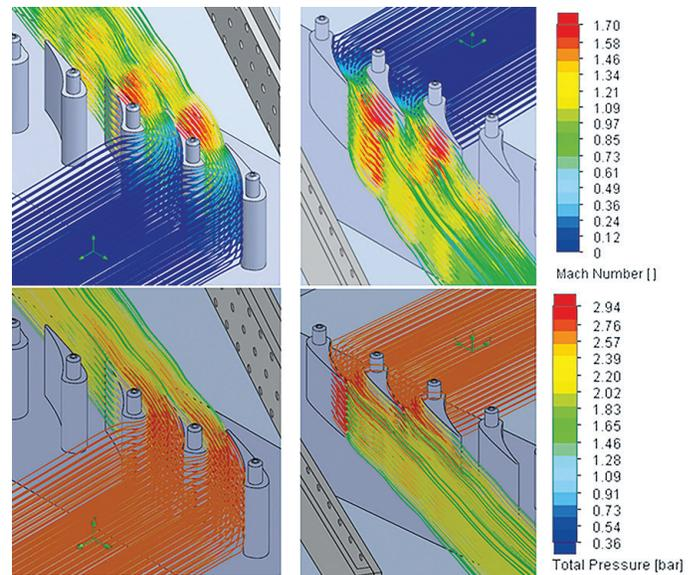
Figure 9: Mach number (top) and total pressure (bottom) distribution in the streamlines.
