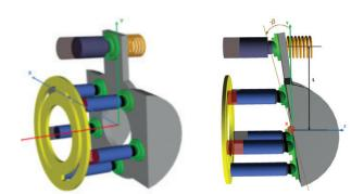
The pump model has been automatically generated and parametrized importing the CAD file directly into Simcenter Amesim. Additionally, the control valve, stroking piston and swash plate mechanics have been added to realize the swash plate regulation to reduce the pump displacement when the delivery pressure reaches the value equivalent to a spring preload.
