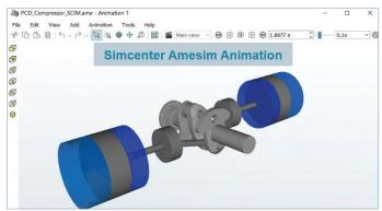
The current Simcenter Amesim application shows a dual-acting compressor with two stages and two heat exchangers (inter and after-cooler) for temperature cooling.
