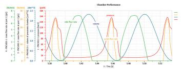
At the outlet of each compression stage users can verify the temperature level, pressure pulsations and the influence of pneumatic lines on the damping or amplification of these oscillations.
