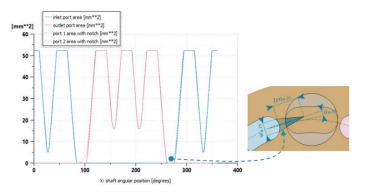
As soon as the pump drawing is available, the CAD import capabilities allow the user to automatically generate the sketch and parametrize the pump model by directly retrieving its geometry.
