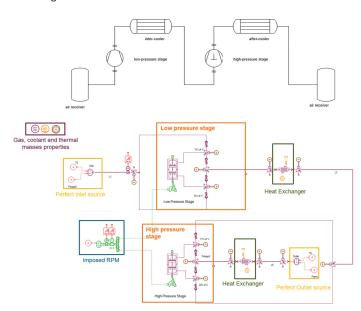
The above simulation model allows the user to improve the compressor performance by predicting torque demand, understanding gas line dynamics, reducing pumping losses (friction, leakage) and improving the compressor driveline dynamics (modal shapes, frequency response). Simcenter Amesim enables users to evaluate the performance of each chamber in terms of volume variation, inlet and outlet flowrates and internal pressure.
