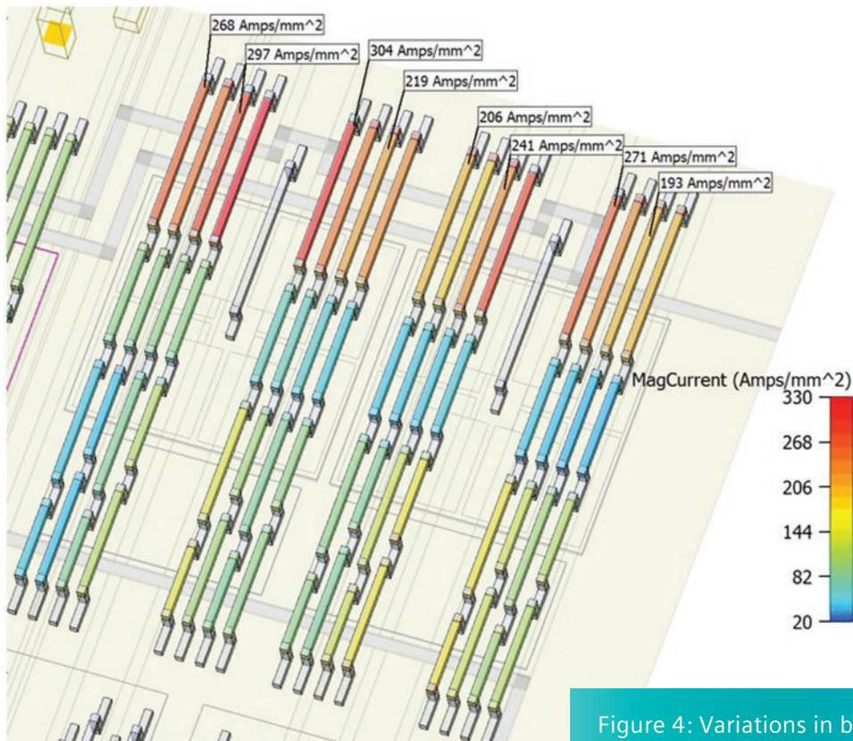
Figure 4: Variations in bond wire current fluxes.
