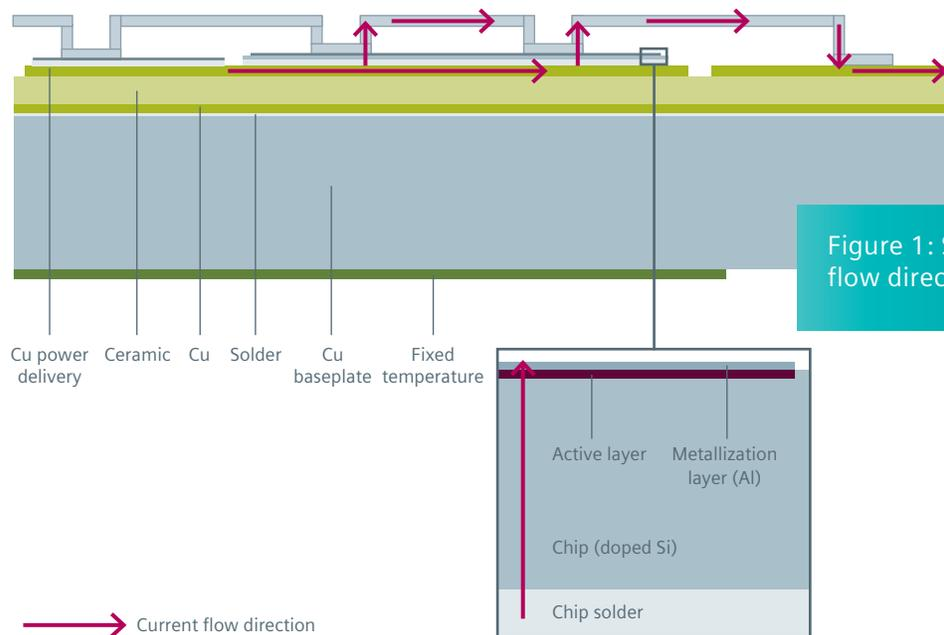
Figure 1: Stackup and current flow direction.
