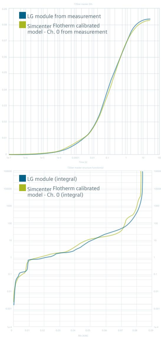
Figure 2:  $Z_{th}$  and cumulative structure function calibration comparison.
