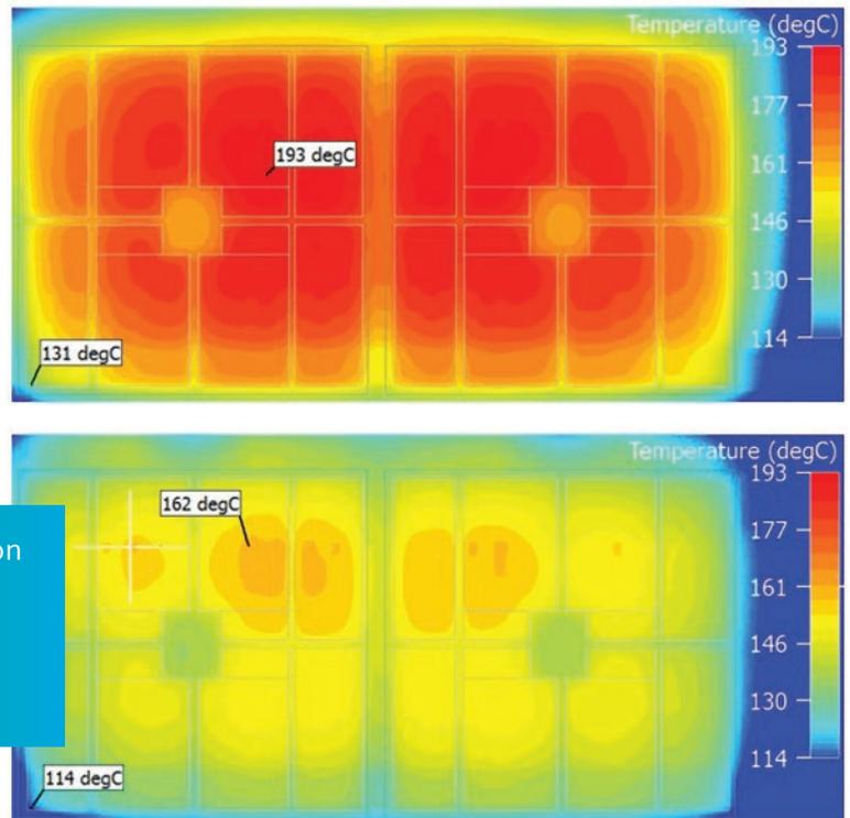
Figure 5: Temperature prediction with full power uniformly dissipated (top) and with an electrothermal approach (bottom).
