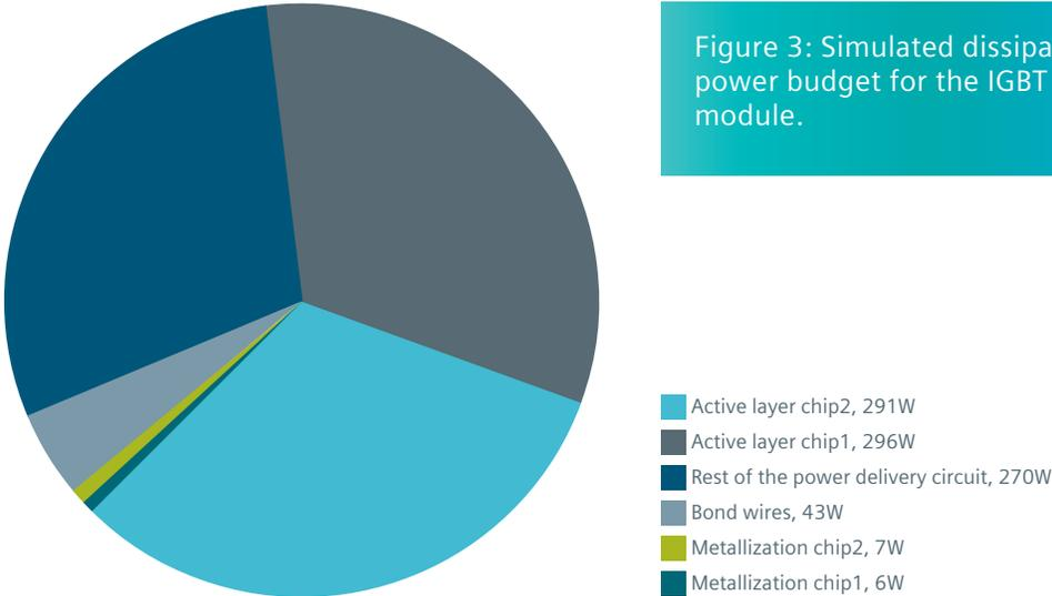
Figure 3: Simulated dissipated power budget for the IGBT module.
