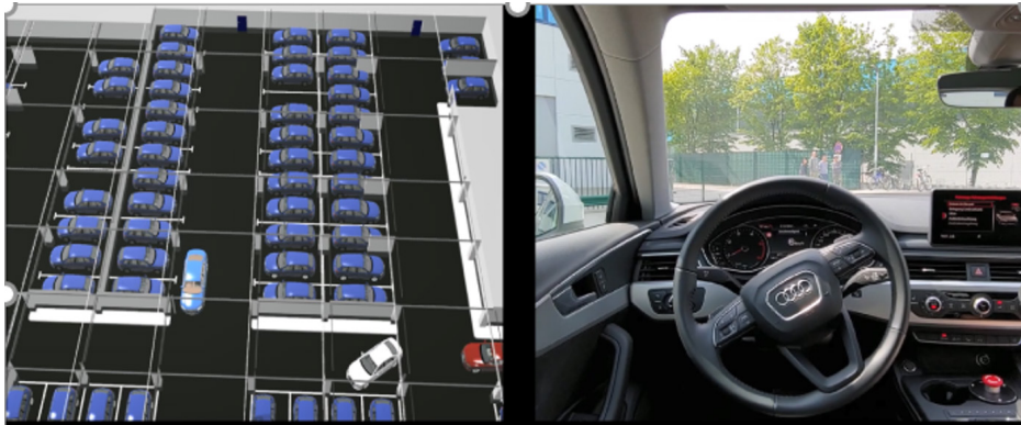
Mixed-reality experiment with a physical vehicle and virtual static/dynamic actors (*).
