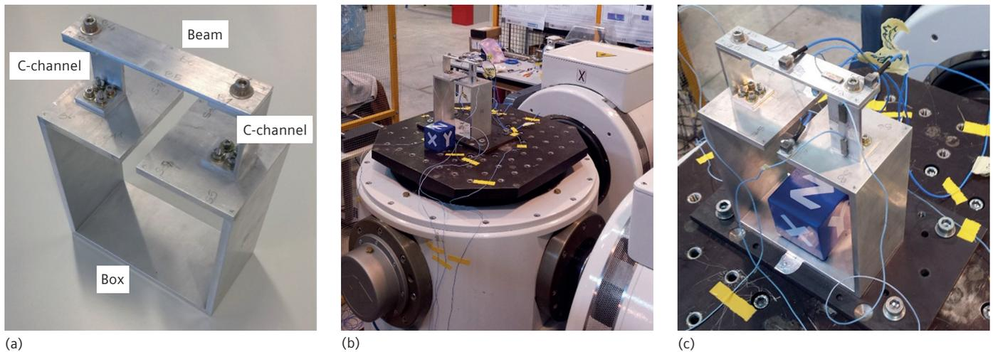
Figure 2: BARC structure (a). Test setup with BARC mounted on the three-axis shaker at the University of Ferrara (b). Accelerometers and strain sensors on the unit being tested (c).
