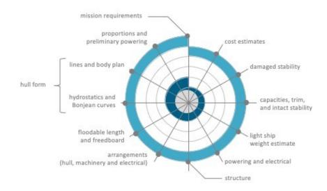
are met. For example, once the initial or concept phase is complete for hull form, the process moves on to preliminary or contract design, and so on. The spiral repeats for each requirement and through each phase.
