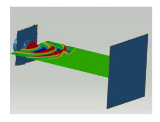
Ultrasonic 40 kHz pulse simulation
