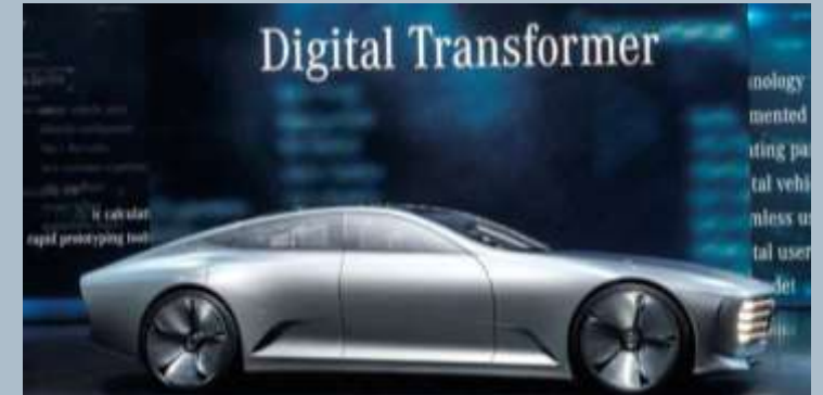
Vehicle changes shape over 80 km/h to reduce drag at highway speeds
