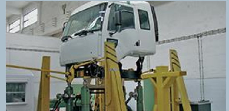
Cabin rig test to represent 1.2 million kilometers
