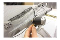
without external support or the need for alignment. Thanks to the patented internal suspension, the inert mass is dynamically decoupled from the test object and the force is always aligned along the internal stinger axis. This significantly improves the efficiency of testing by eliminating the support and alignment work associated with conventional shaker testing. Additionally, you only need one operator to execute data acquisition.
