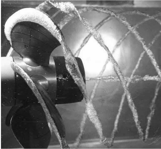
Figure 4: Tip vortex and blade back cavitation (left), and cavitation damage (right).
