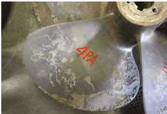
Propeller with cavitation damage.
