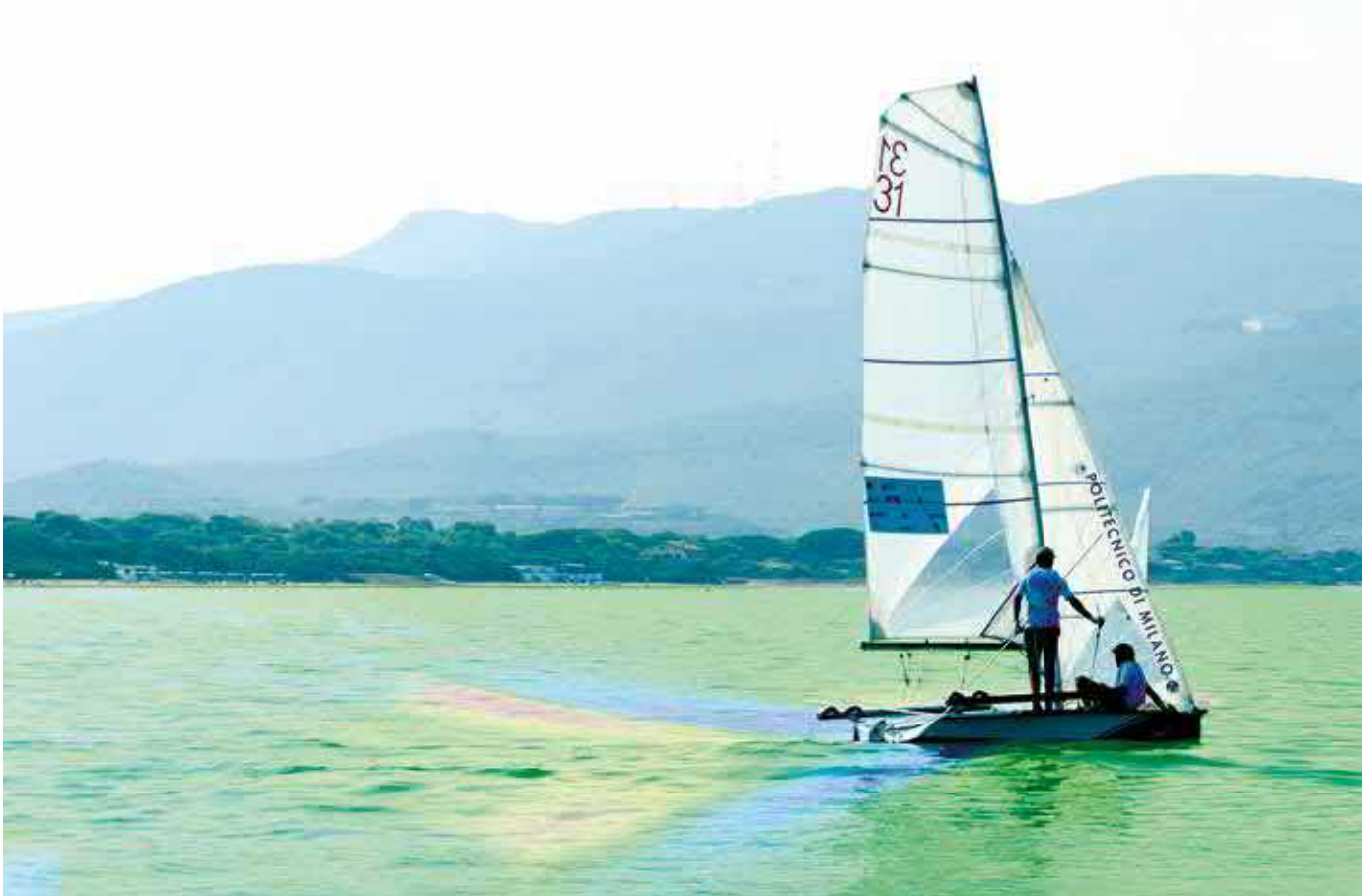
Figure 1: A photograph of the R3 skiff sailing upwind and the overlaid results of the hydrodynamic simulations.
