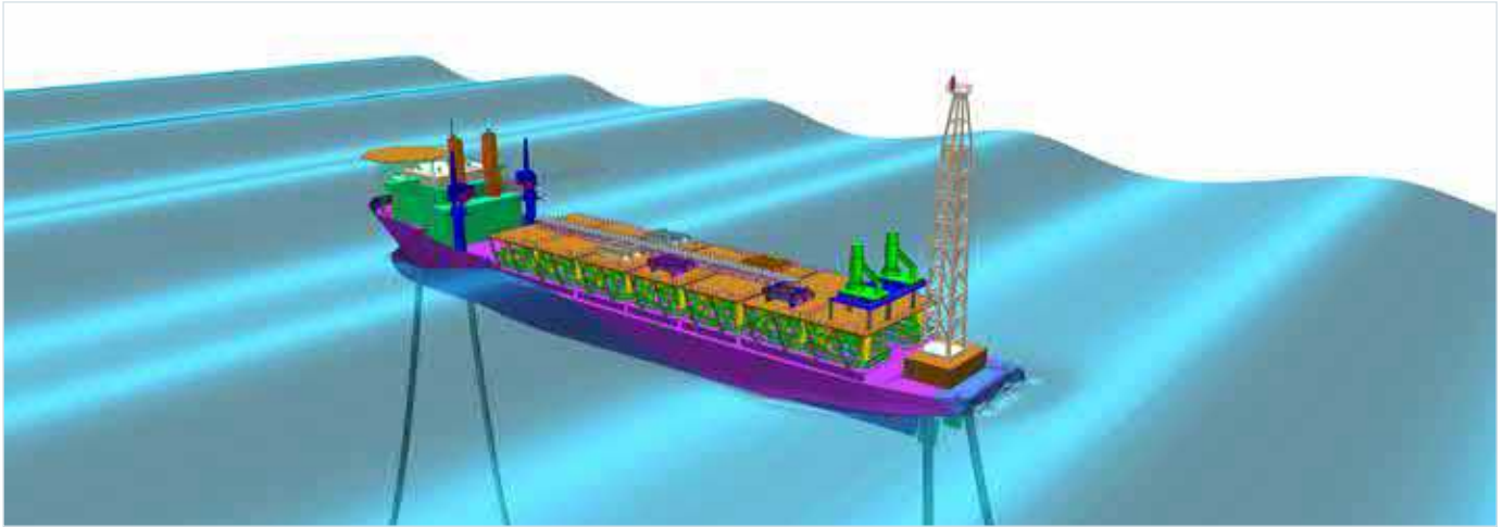
Simcenter STAR-CCM+ also includes a number of wave models that can be used to test the performance of a vessel under a range of realistic sea states.
