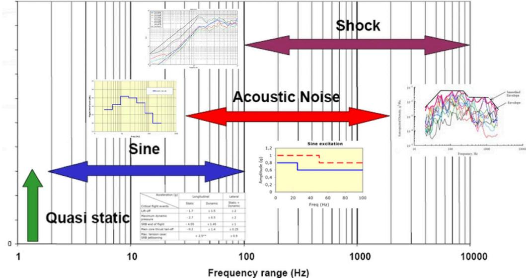
Figure 2. Vibration environments and corresponding frequency ranges.
