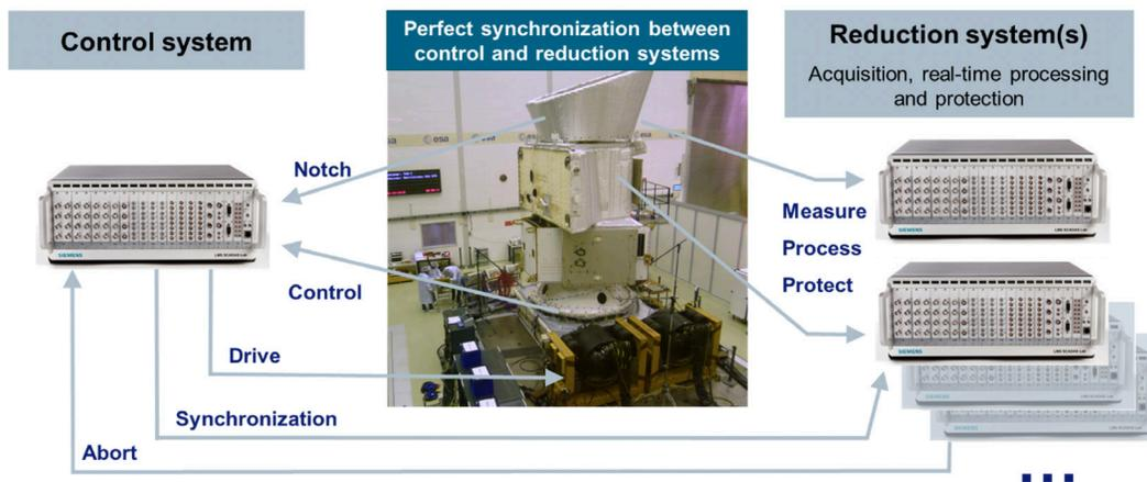
Figure 7. Set up with control and reduction system.
