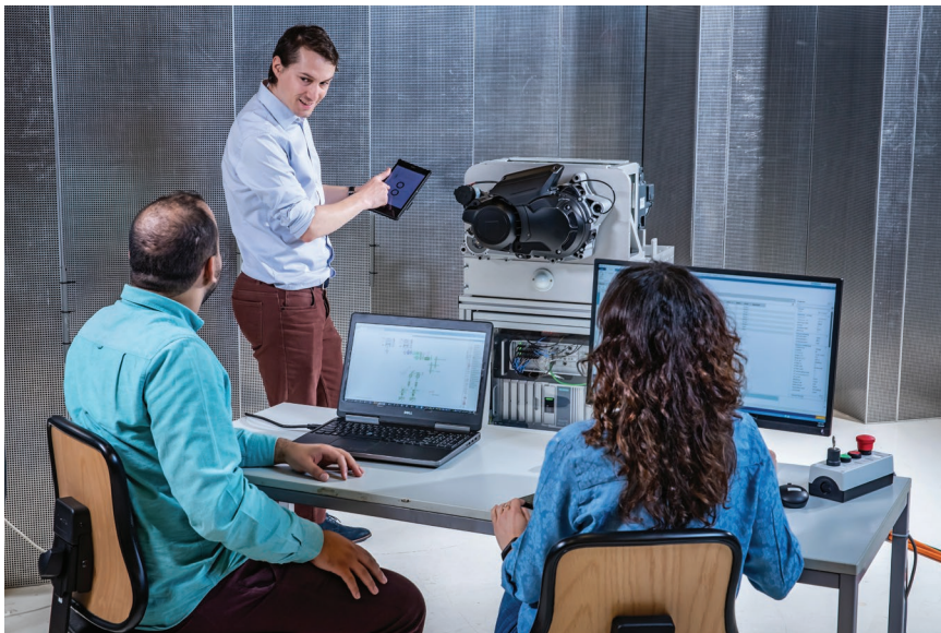
Figure 5. Front-loading of motorcycle gearbox testing. From proving ground to bench testing in near real-life conditions via the system-in-the-loop approach.
