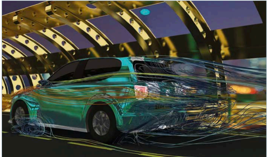
Figure 7. Simcenter STAR-CCM+ for vehicle aerodynamics optimization.
