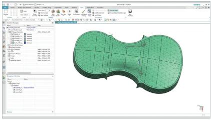
different issues of stringed instruments. The project that Professor Ravina leads is oriented towards testing the vibrations and acoustical responses of instruments.
