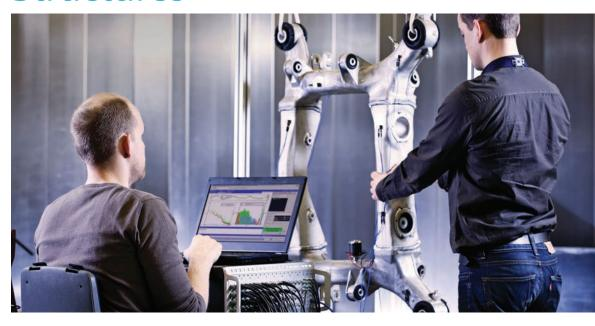
Simcenter Testlab Structures is a comprehensive suite of structural dynamics and modal testing and analysis software. Characterizing the structural dynamics of a structure used to be a long and complex process involving extensive trial-and-error and time-consuming test setups. This is no longer the case. With Simcenter Testlab Structures and the Simcenter SCADAS system, it's easier to perform large-scale modal surveys – in hours rather than days.
