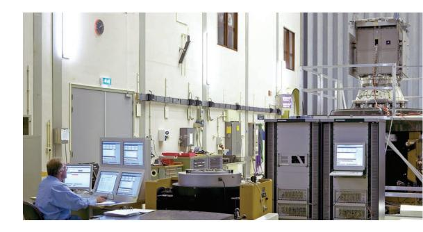
Simcenter Testlab Environmental provides you with a powerful, high-speed multichannel vibration control system for dynamic environmental testing, certified for spacecraft testing. The vibration control systems can be expanded to hundreds of control, measurement and limiting channels. The solution is easy to use for routine random, shock, sine and combined modes testing and has everything you need for state-of-the-art control and extensive data analysis.
