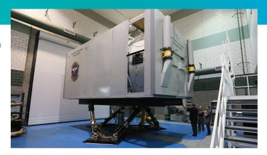
electronic actuation products are used for flight simulation, ground vehicle simulation and the entertainment industry.
