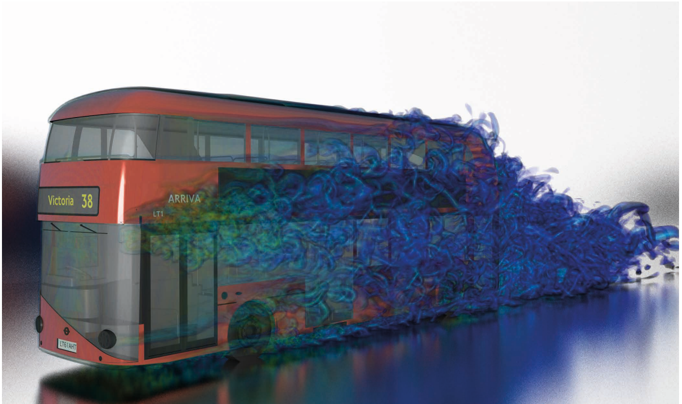
Aerodynamic analysis of the new transport bus in London with STAR-CCM+.
