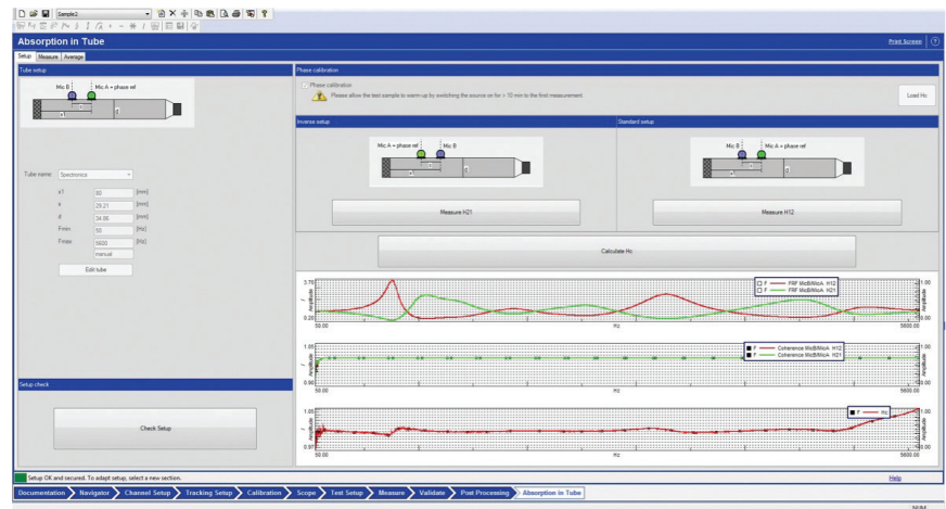
Step-by-step measurement of sound absorption using Simcenter Testlab.
