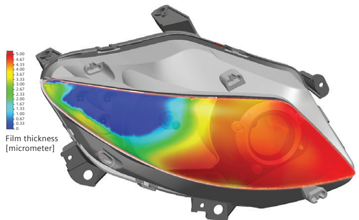
Figure 9: CAD-embedded automotive headlight simulation for transient defogging analysis.
