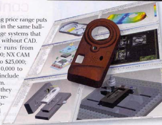
◀ Figure 2: This figure shows all of the applications that are available in Pro/E CAM for mold maker: design, detailing of mold base, creation of mold base, core/cavity creation, NC toolpath generation, and plastic injection analysis.
