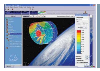
The conduction, which can either be isotropic or orthotropic, can depend on the temperature and time. The heat transfer capacity behavior of the material can be modeled as a function of temperature or by the use of an enthalpy formulation. This formulation is used to accurately integrate a phase change (presence of latent heat) process without major restrictions on the time step size.
