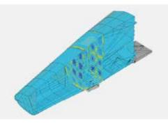
Results are postprocessed graphically in the form of curves (time-wise evolution of a value) as iso-values (temperature at given instant) or as animations.
