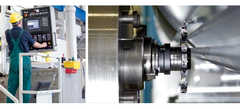
Siemens PLM Software's unique combination of technology also provides great value for the end users of the machine tools. The virtual machine can be used for many nonproductive tasks, such as program testing, setup checking and even operator training. Program code can be edited and changes verified right on the virtual machine, saving valuable time on the real machine.
