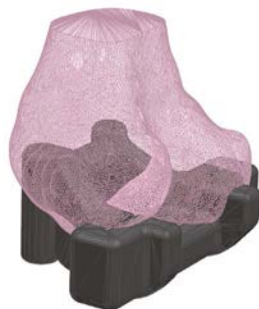
Convergent modeling: facet model of knee joint with b-rep surgical guide, modeled in single architecture.
