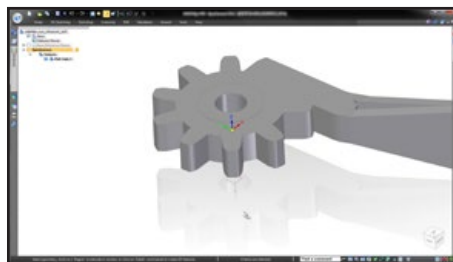
2 Start by importing the part geometry. Our example is from another system, so you have no feature information, which would traditionally mean a lot of redesign work
