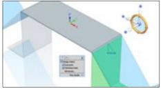
**DESIGN INTENT:** Design Intent in Synchronous Technology is stored right on the model, rather than indirectly in the sketches. A set of filters and face selection criteria allow you to enforce relationships such as parallelism and dimensional constraints, or easily remove them to change the design intent and make edits to your model.
