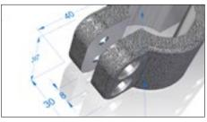
**3D DIMENSIONS:** History-based systems require dimensions to build geometric features individually. With Synchronous Technology, dimensions can be placed in 3D space to define real world relationships, rather than having to define them just to derive features. And it works as well on third party data as it does with
