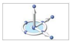
**STEERING WHEEL:** Like in your car, this is the main control of Synchronous Technology. This gives you control over translation, rotation, and scaling of the faces you have selected. It can be dragged, dropped and snapped to axial positions to allow precise manipulation. Combined with Design Intent (see the panel to the right) it gives you control over your model.
